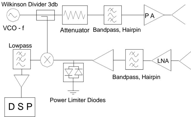
**Figure 10.** Block diagram of 2.45 GHz radar system (SOZON III).
