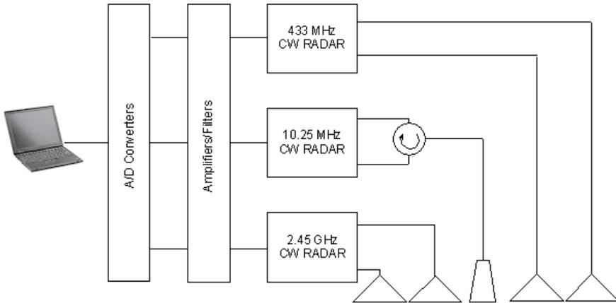
**Figure 3.** Schematic diagram of the three-band frequency CW-Doppler radar (the complete system SOZON II).
