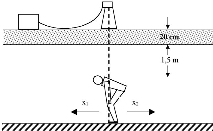
**Figure 14.** Schematic of the measurement procedure followed throughout the Life Detector Radar systems' testings.
