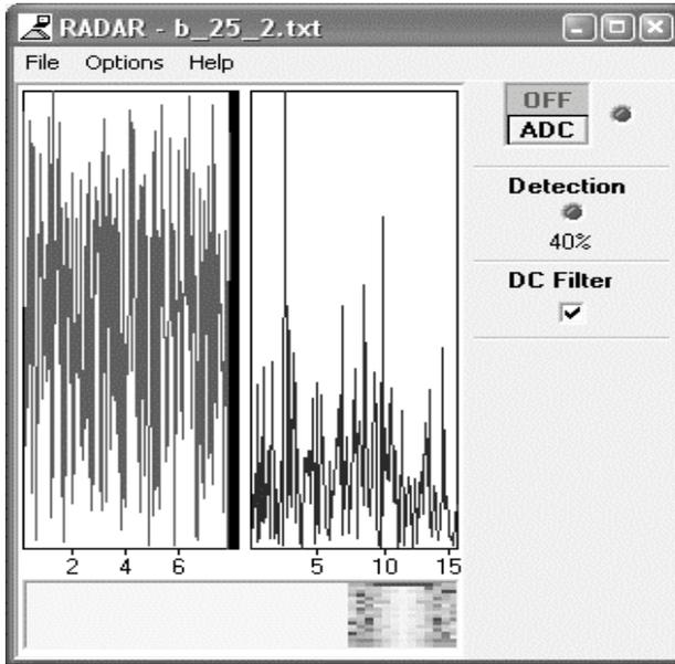
**Figure 1.** Screenshot of the user interface. Apart from the time domain signal and the FFT, there is also a display of the detection probability, as well as a “history file” at the bottom side of the graphs for keeping the previous measurements.
