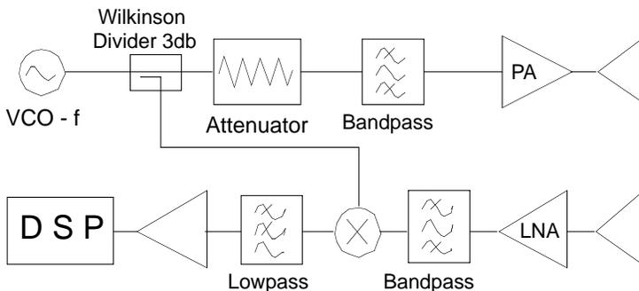
**Figure 2.** System block diagram of life detector for the lower frequencies of 433 MHz and 2.45 GHz consisting of three parts: antenna part, microwave circuit part and low frequency part.
