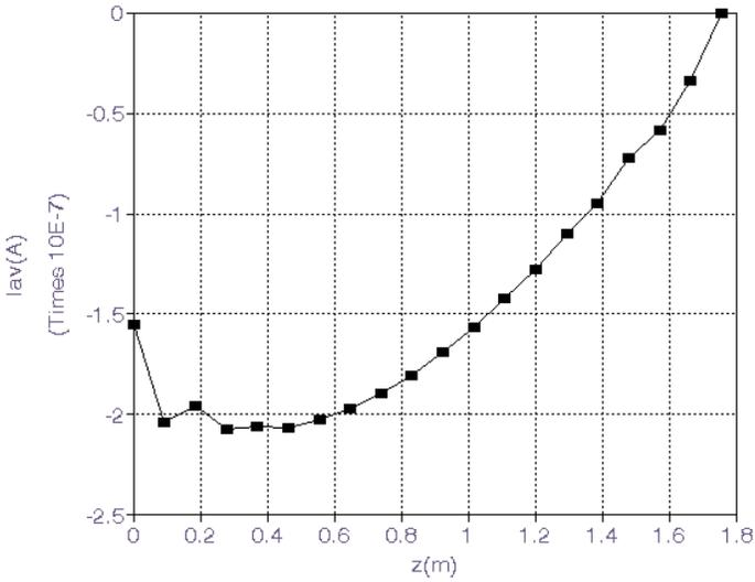
**Figure 3.** Spatial distribution of average values of the transient current due to the Gaussian pulse exposure.
