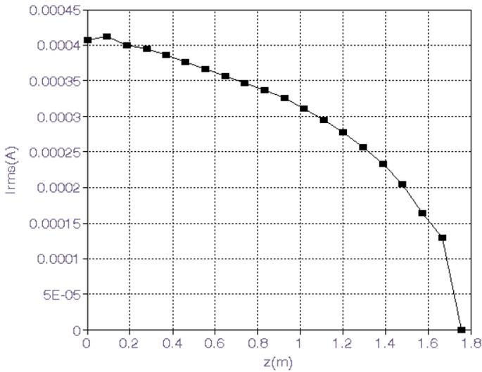
**Figure 4.** Spatial distribution of average values of the transient current due to the Gaussian pulse exposure.
