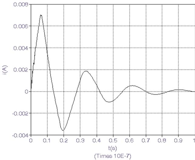
**Figure 7.** Transient current induced in the feet due to the step function exposure.
