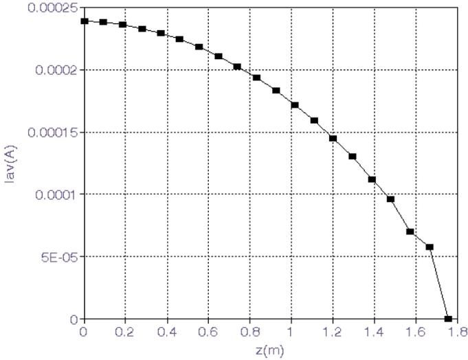
**Figure 13.** Spatial distribution of average values of the transient current due to the EMP exposure.
