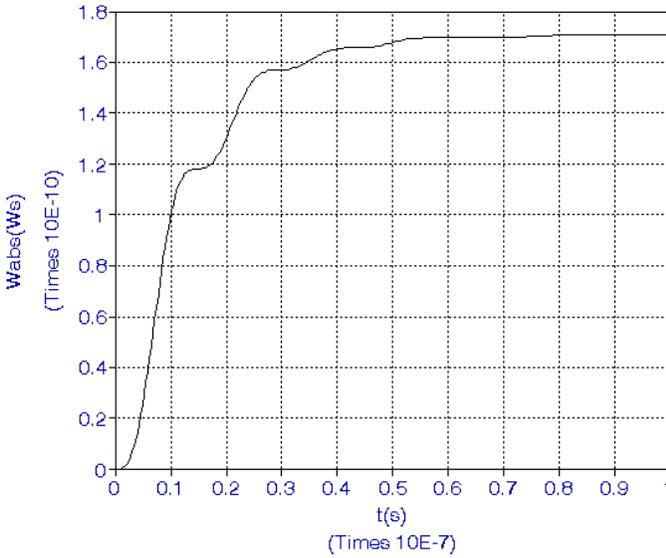
**Figure 16.** Total energy absorbed in the body due to the EMP exposure.
