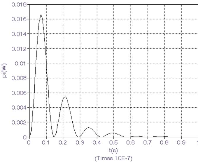
**Figure 15.** Instantaneous power dissipated within the body due to the EMP exposure.
