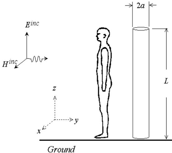
**Figure 1.** Cylindrical model of the human body exposed to a vertically polarized transient field.
