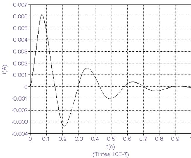
**Figure 12.** Transient current induced in the feet due to the EMP exposure.
