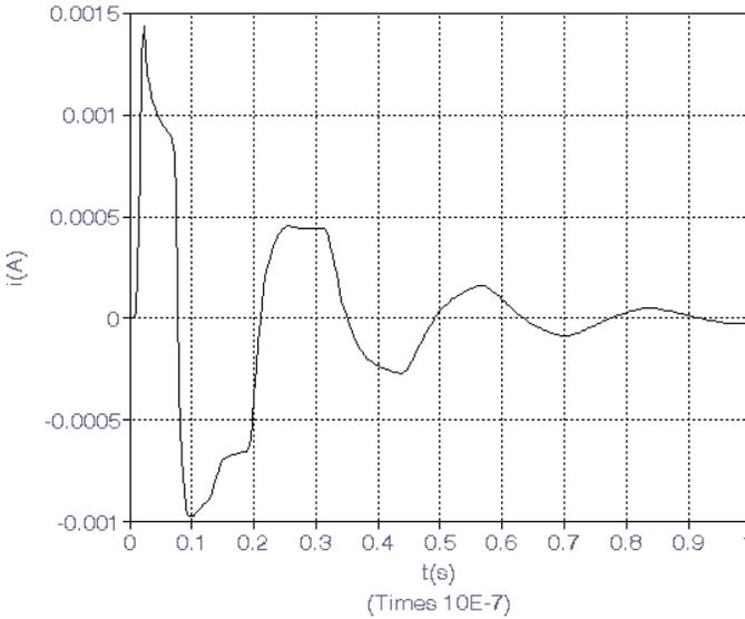
**Figure 2.** Transient current induced in the feet due to the Gaussian pulse exposure.
