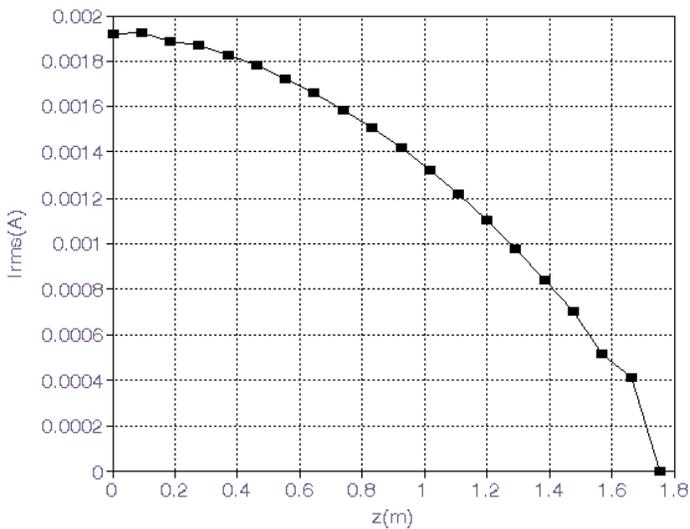
**Figure 9.** Spatial distribution of *rms* values of the transient current due to the step exposure.
