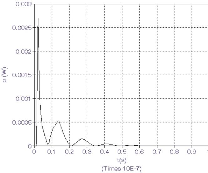
**Figure 5.** Instantaneous power dissipated within the body due to the Gaussian pulse exposure.
