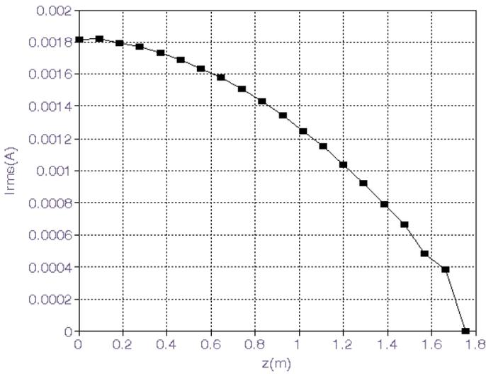
**Figure 14.** Spatial distribution of *rms* values of the transient current due to the EMP exposure.
