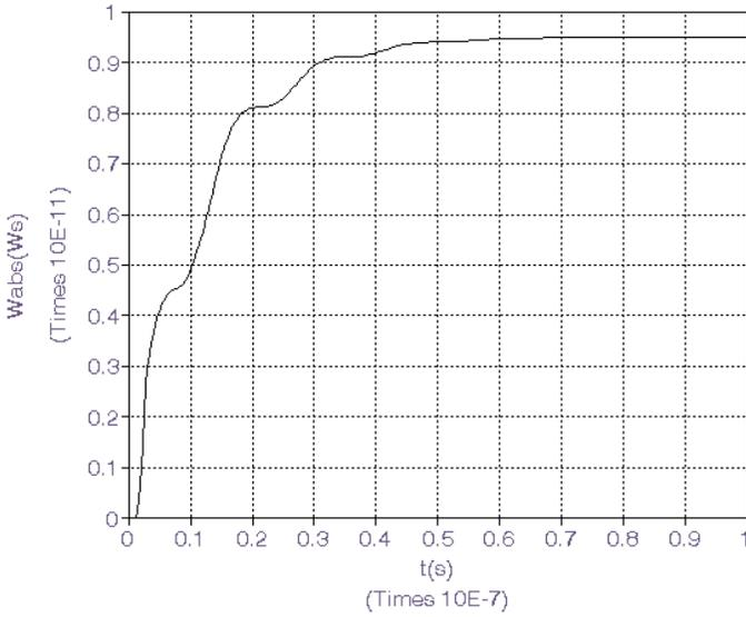
**Figure 6.** Total energy absorbed in the body due to the Gaussian pulse exposure.
