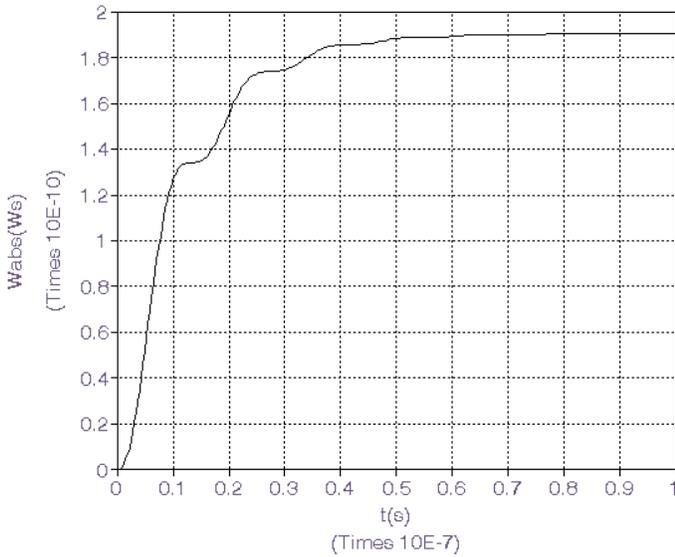
**Figure 11.** Total energy absorbed in the body due to the step exposure.
