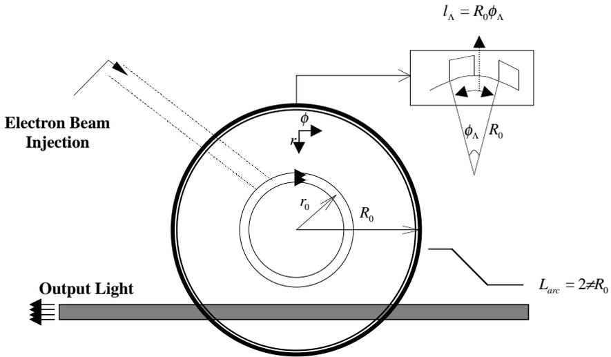
**Figure 1.** 2-dimensional model for the electro-optical modulator.
