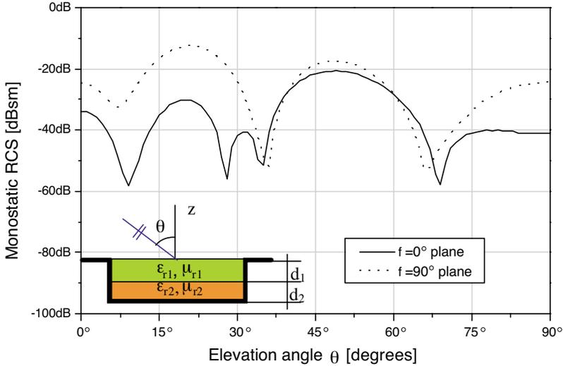
**Figure 5.** Monostatic RCS  $\sigma_{\theta\theta}$  for a  $\varphi$ -polarized incident plane wave at  $f = 10$  GHz. The cavity dimensions are:  $10 \text{ cm} \times 10 \text{ cm} \times 1.5 \text{ cm}$ ; while the slab parameters are:  $d_1 = 1.02 \text{ cm}$ ,  $d_2 = 1.02 \text{ cm}$ ,  $\epsilon_{r1} = 9.957$ ,  $\mu_{r1} = 0.037$ ,  $\epsilon_{r2} = 5.747$ ,  $\mu_{r2xx} = \pm 0.283$ ,  $\mu_{r2yy} = -0.283$ ,  $\mu_{r2zz} = 0.283$ .
