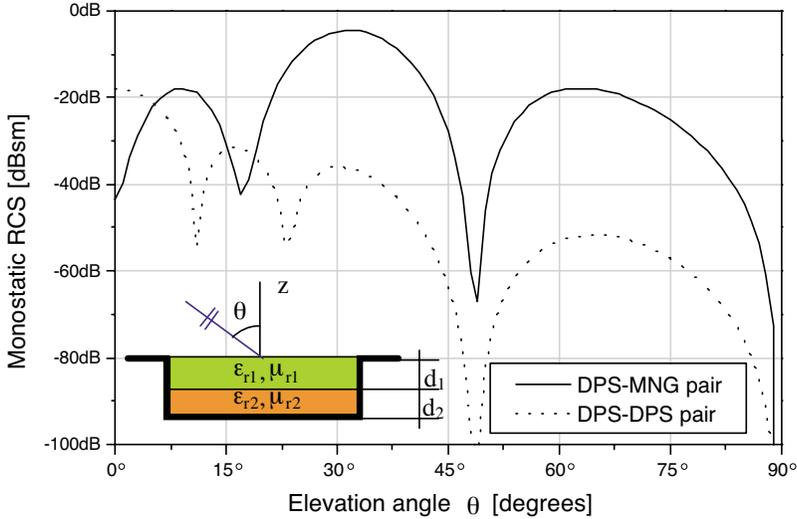
**Figure 3.** Monostatic RCS  $\sigma_{\theta\theta}$  at  $f = 10$  GHz for a  $\theta$ -polarized incident plane wave. The cavity dimensions are:  $10 \text{ cm} \times 10 \text{ cm} \times 1.5 \text{ cm}$ ; while the slab parameters are:  $d_1 = 1.02 \text{ cm}$ ,  $d_2 = 1.02 \text{ cm}$ ,  $\epsilon_{r1} = 9.957$ ,  $\mu_{r1} = 0.037$ ,  $\epsilon_{r2} = 5.747$ ,  $\mu_{r2} = \pm 0.283$ .
