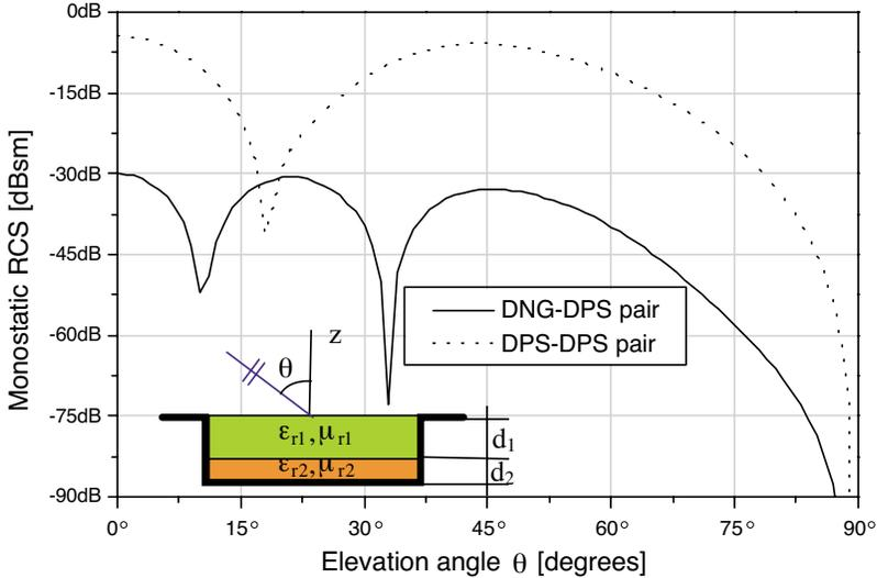
**Figure 2.** Monostatic RCS  $\sigma_{\theta\theta}$  at  $f = 5$  GHz for a  $\theta$ -polarized incident plane wave. The cavity dimensions are:  $10 \text{ cm} \times 10 \text{ cm} \times 1.5 \text{ cm}$ ; while the slab parameters are:  $d_1 = 1 \text{ cm}$ ,  $d_2 = 0.5 \text{ cm}$ ,  $\epsilon_{r1} = \pm 2$ ,  $\mu_{r1} = \pm 1$ ,  $\epsilon_{r2} = 4$ ,  $\mu_{r2} = 2$ .
