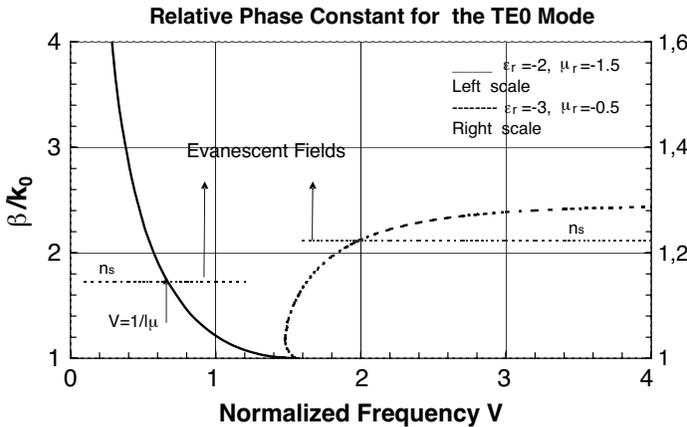
**Figure 6.** The phase constant of the dominant TE<sub>0</sub> mode on a BW slab with  $n_s \equiv \sqrt{\epsilon_r \mu_r} > 1$  and  $|\mu_r| > 1$  (solid curve) and  $n_s \equiv \sqrt{\epsilon_r \mu_r} > 1$  and  $|\mu_r| < 1$  (dotted curve).
