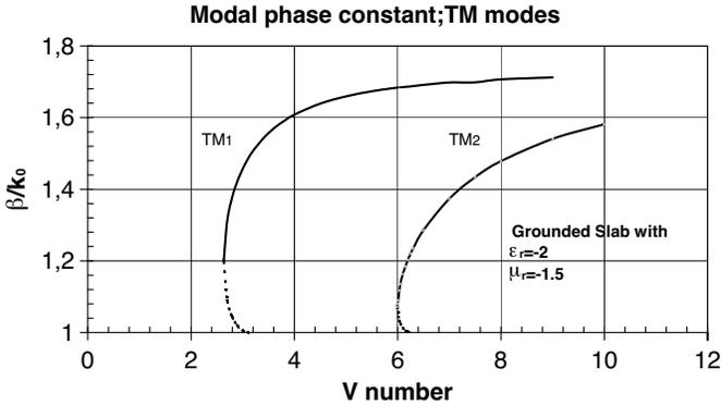
**Figure 2.** Relative phase constant of TM modes versus normalized frequency  $V$ .
