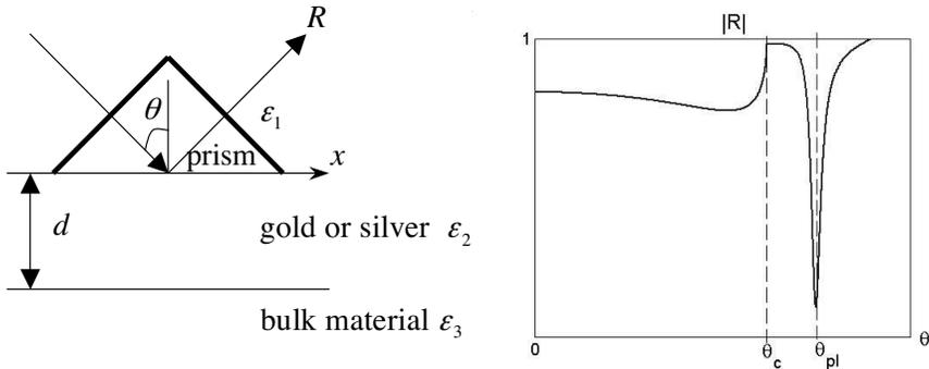
**Figure 2.** Surface plasmon geometry and the reflection coefficient plot of a conventional optical surface plasmon sensor  $\varepsilon_1 = 2.25$ ,  $\varepsilon_2 = -10 - j0.1$ ,  $\varepsilon_3 = 1.75$ ,  $\mu_1 = \mu_2 = \mu_3 = 1$ ,  $d = 0.05 \mu\text{m}$ ,  $\lambda = 0.6 \mu\text{m}$ .
