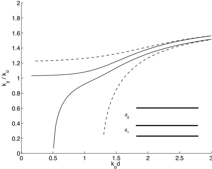
**Figure 3.** Slow-wave factor  $k_y/k_0$  versus  $k_0d$ , calculated for  $d_2/d_1 = 5$  (solid curves) and  $d_2/d_1 = 0.5$  (dashed curves). The wires are directed along  $y$ -axis. Parameters of the wire slab are the same as in Figure 2. Dispersion of the two lowest-order modes is shown.
