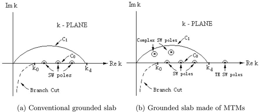
**Figure 2.** Surface wave poles in  $k$ -plane.
