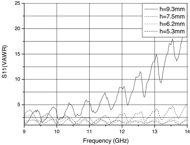
**Figure 5.** Measured  $S_{11}$  of monopoles of different length in Medium-2 (strips only).
