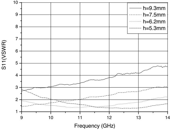
**Figure 3.** Measured  $S_{11}$  of monopoles of different length in the Air.
