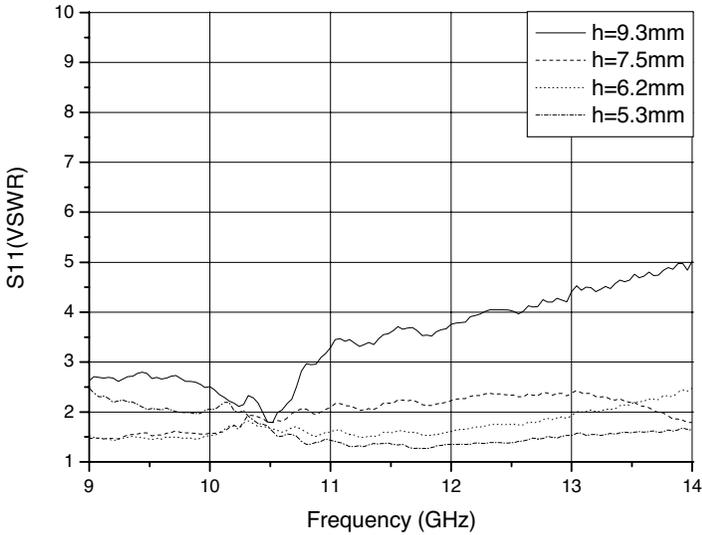
**Figure 4.** Measured  $S_{11}$  of monopoles of different length in Medium-1 (SRRs only).
