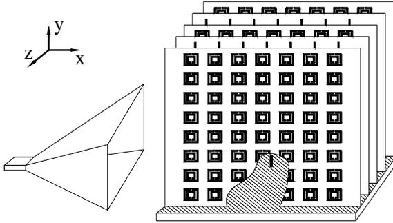
**Figure 2.** Experiment setup of monopole in meta-material.
