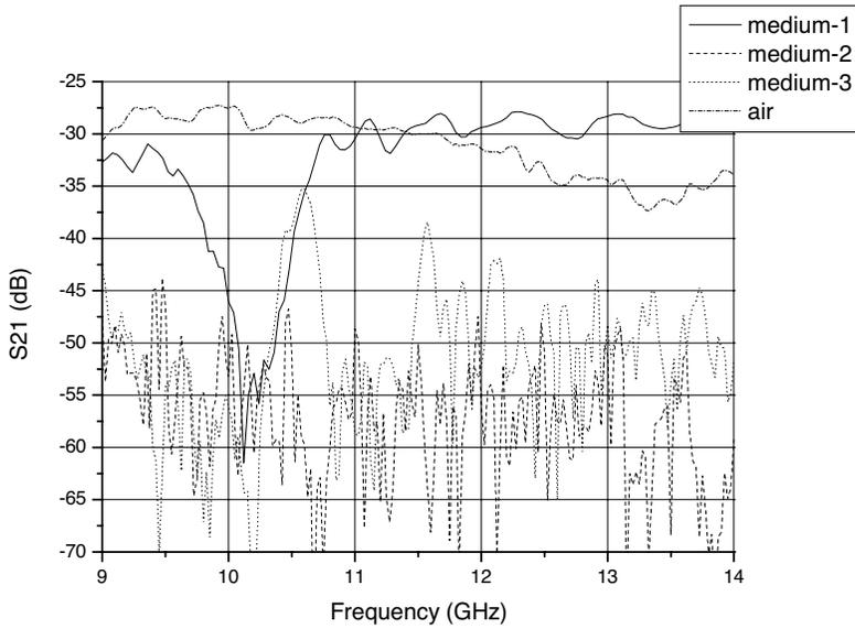
**Figure 7.** Measured  $S_{21}$  of  $h = 7.5$  mm monopoles in different media.
