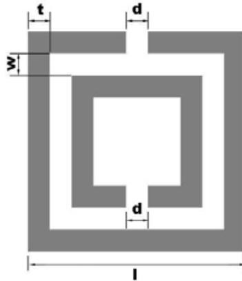
**Figure 1.** Single SRR with parameters  $l = 3$  mm,  $d = t = w = 0.3$  mm.
