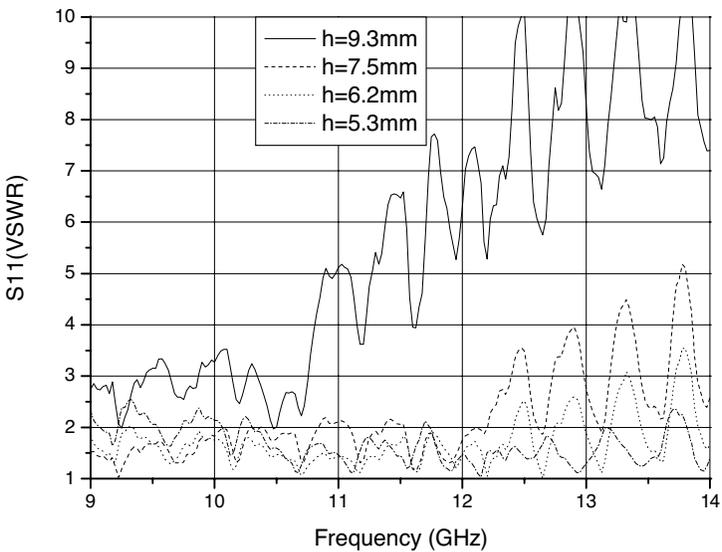
**Figure 6.** Measured  $S_{11}$  of monopoles of different length in Medium-3 (SRRs & strips).
