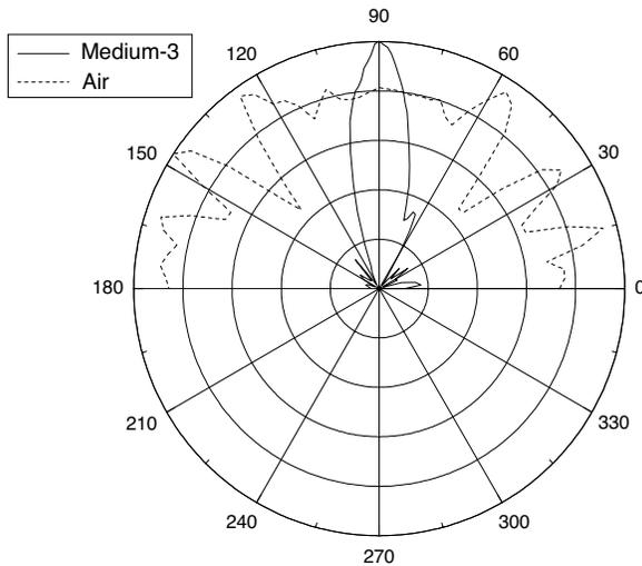
**Figure 9.** Normalized field pattern of 10.6 GHz.
