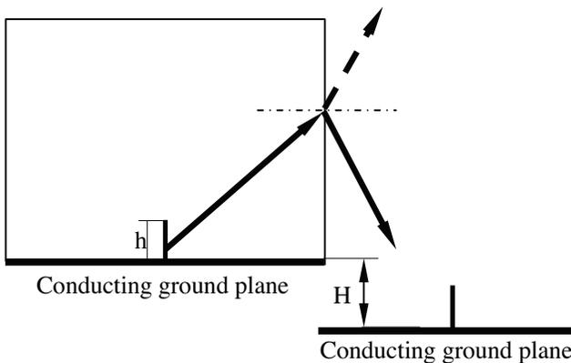
**Figure 10.** Experimental setup for refraction received by monopole.
