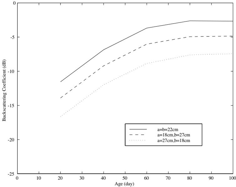
**Figure 6.** Simulated temporal variation of the L-band backscattering returns assuming the looking direction of the radar to be the  $x$ -direction. Simulated cases include fields with equal spacing between rice plants ( $a = b = 22$  cm), fields with spacings  $a = 18$  cm and  $b = 27$  cm, and fields with spacings  $a = 27$  cm and  $b = 18$  cm.
