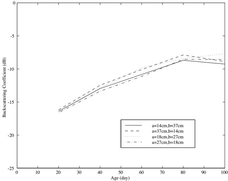
**Figure 7.** Simulated temporal variation of the C-band backscattering returns assuming the looking direction of the radar to be the  $x$ -direction. Simulated cases include fields with spacings  $a = 14$  cm and  $b = 37$  cm, fields with spacings  $a = 37$  cm and  $b = 14$  cm, fields with spacings  $a = 18$  cm and  $b = 27$  cm, and fields with spacings  $a = 27$  cm and  $b = 18$  cm.
