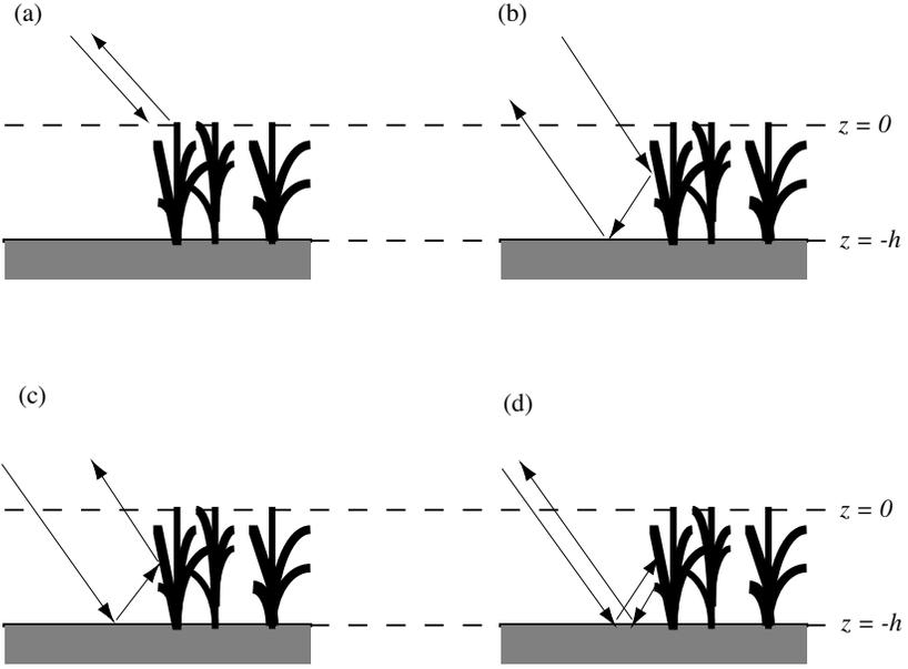
**Figure 2.** Four major scattering mechanisms in the rice canopy: (a) direct scattering from scatterers, (b) single scattering from the scatterer followed by reflection off the boundary, (c) surface scattering followed by single scattering, (d) reflection by the boundary followed by single scattering from the scatterer and further followed by reflection off the boundary.
