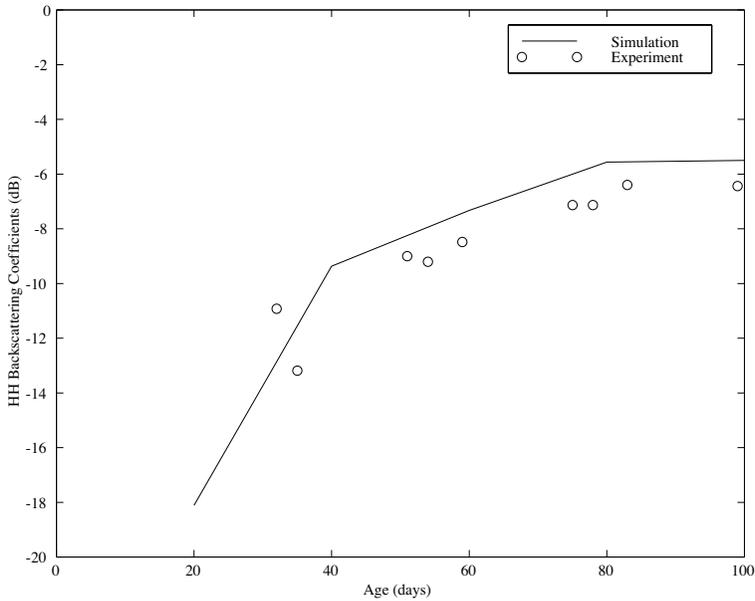
**Figure 3.** Comparison between the simulated HH backscattering coefficients and RADARSAT data as a function of rice age. The frequency is at C-band and the incident angle is  $23^\circ$ .
