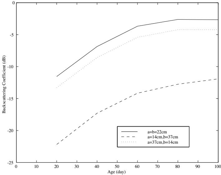
**Figure 5.** Simulated temporal variation of the L-band backscattering returns assuming the looking direction of the radar to be the  $x$ -direction. Simulated cases include fields with equal spacing between rice plants ( $a = b = 22$  cm), fields with spacings  $a = 14$  cm and  $b = 37$  cm, and fields with spacings  $a = 37$  cm and  $b = 14$  cm.
