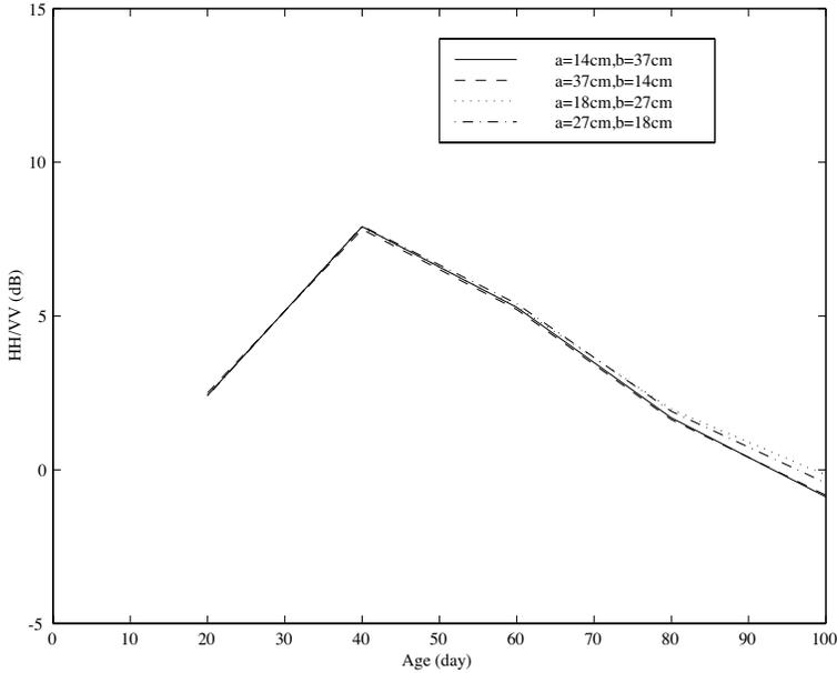
**Figure 8.** Simulated temporal variation of the ratio of L-band copol backscattering coefficients, HH over VV, assuming the looking direction of the radar to be the  $x$ -direction. Simulated cases include fields with spacings  $a = 14$  cm and  $b = 37$  cm, fields with spacings  $a = 37$  cm and  $b = 14$  cm, fields with spacings  $a = 18$  cm and  $b = 27$  cm, and fields with spacings  $a = 27$  cm and  $b = 18$  cm.
