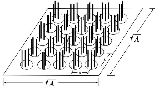
**Figure 1.** Configuration for the scattering model from a rice field. Rice plants are planted with spacing  $a$  in the  $x$  direction and spacing  $b$  in the  $y$  direction over a square area  $A$ . Within a rice bunch, the stems are randomly placed inside a circle with uniform distribution.
