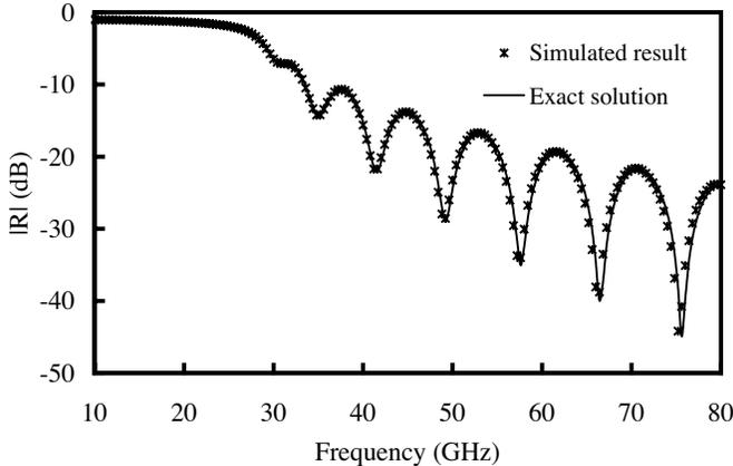
**Figure 1.** Comparison of reflection coefficient magnitude simulated using (FD)<sup>2</sup>TD method with the analytical solution.
