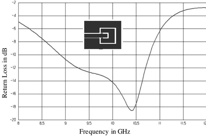
**Figure 8.** Return loss for two switches in CPW.
