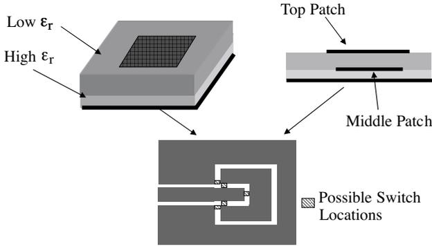
**Figure 2.** Proposed antenna configuration using loop/slot coupling.
