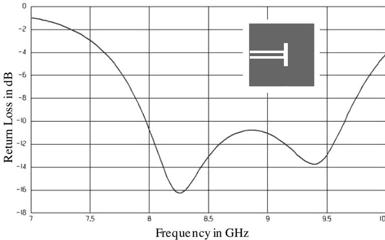
**Figure 3.** Return loss for capacitive slot coupling.
