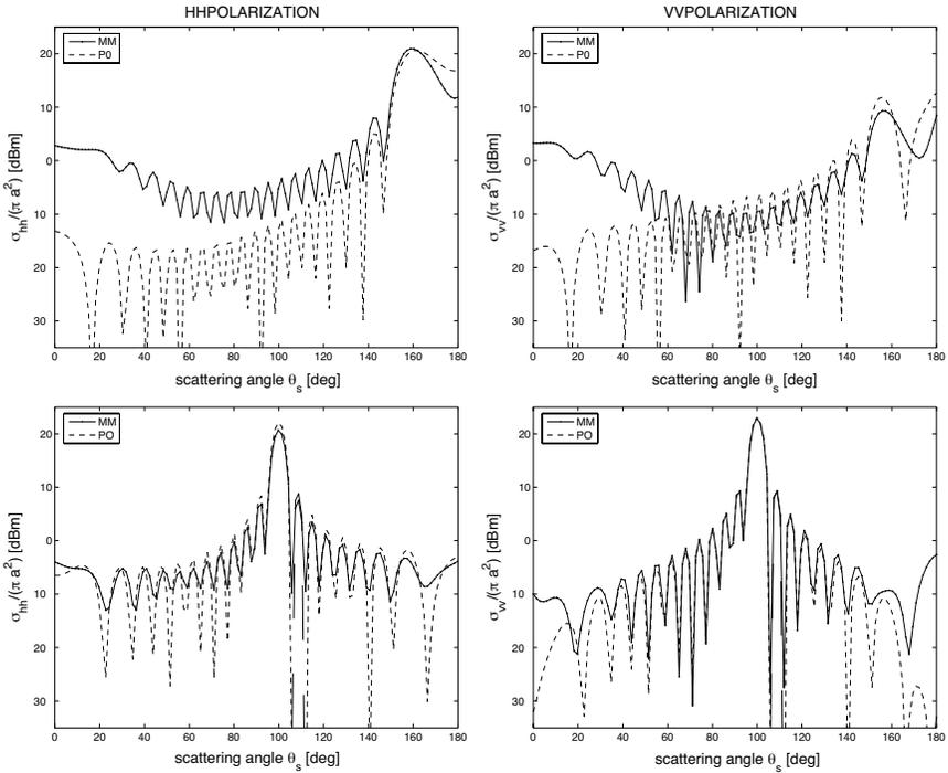
**Figure 6.** Normalized bistatic scattering coefficient vs. scattering angle for finite dielectric cylinder with  $L = 10.0\lambda$ ,  $a = 0.4\lambda$ ,  $\varepsilon_r = 18j6$ , and incident angle  $\theta_i = 20^\circ$  (top) and  $\theta_i = 80^\circ$  (bottom).
