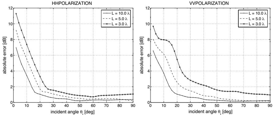
**Figure 8.** Absolute error vs. incident angle for finite dielectric cylinder with  $a = 0.4\lambda$ ,  $\varepsilon_r = 18j6$ ,  $L = 10.0\lambda$ ,  $5.0\lambda$ , and  $3.0\lambda$ , for  $hh$ - and  $vv$ -polarization.
