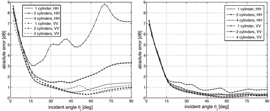
**Figure 11.** Error vs. incident angle for tapered dielectric cylinder with  $L = 10.0\lambda$ , (left)  $a = 0.7\lambda$ ,  $a_2 = 0.1\lambda$ , and (right)  $a = 0.5\lambda$ ,  $b = 0.3\lambda$ . Solid lines are  $hh$ -pol, dashed lines  $vv$ -pol.
