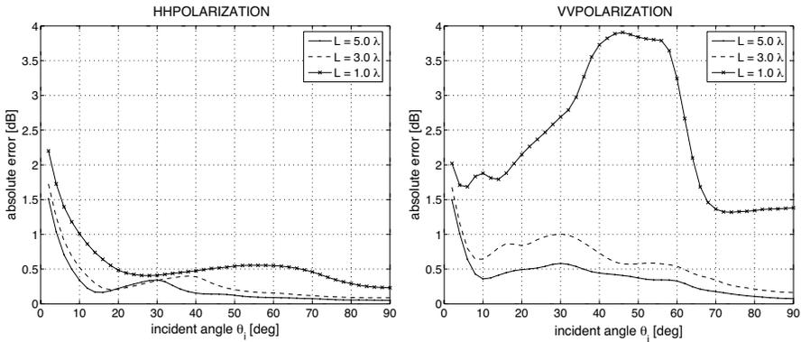
**Figure 7.** Absolute error vs. incident angle for finite dielectric cylinder with  $a = 0.04\lambda$ ,  $\epsilon_r = 18j6$ ,  $L = 5.0\lambda$ ,  $3.0\lambda$ , and  $1.0\lambda$ , for  $hh$ - and  $vv$ -polarization.
