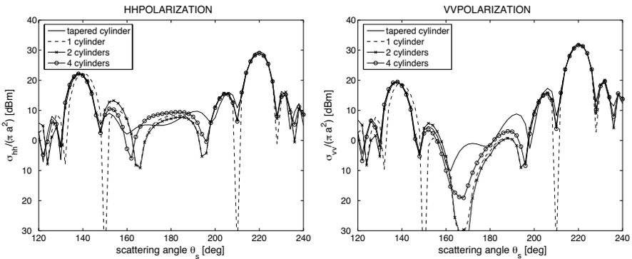
**Figure 10.** Normalized bistatic scattering coefficient vs. scattering angle for tapered dielectric cylinder with  $L = 10.0\lambda$ ,  $a = 0.5\lambda$ ,  $b = 0.3\lambda$ , and incident angle  $\theta_i = 40^\circ$ .  $hh$ - and  $vv$ -polarization (left and right, respectively).
