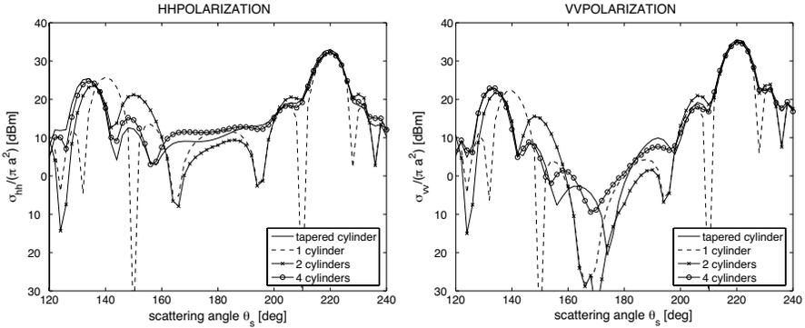
**Figure 9.** Normalized bistatic scattering coefficient vs. scattering angle for tapered dielectric cylinder with  $L = 10.0\lambda$ ,  $a = 0.7\lambda$ ,  $b = 0.1\lambda$ , and incident angle  $\theta_i = 40^\circ$ .  $hh$ - and  $vv$ -polarization (left and right, respectively).
