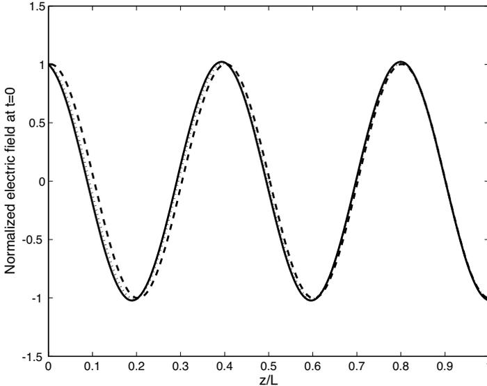
**Figure 5.** Normalized electric field at  $t = 0$  (real part of  $E_x/E_s$ ) for three different values of  $E_s$ . Solid line:  $E_s = 6.87 \times 10^6$  V/m. Dotted line:  $E_s = 12 \times 10^7$  V/m. Dashed line:  $E_s = 22 \times 10^7$  V/m.
