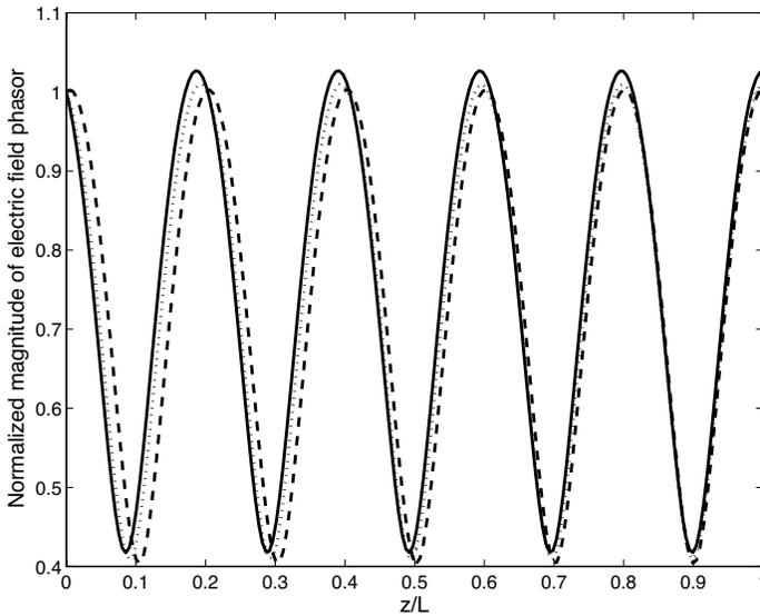
**Figure 4.** Normalized magnitude of electric field phasor,  $|E_x/E_s|$ , for three different values of  $E_s$ . Solid line:  $E_s = 6.87 \times 10^6$  V/m. Dotted line:  $E_s = 12 \times 10^7$  V/m. Dashed line:  $E_s = 22 \times 10^7$  V/m.
