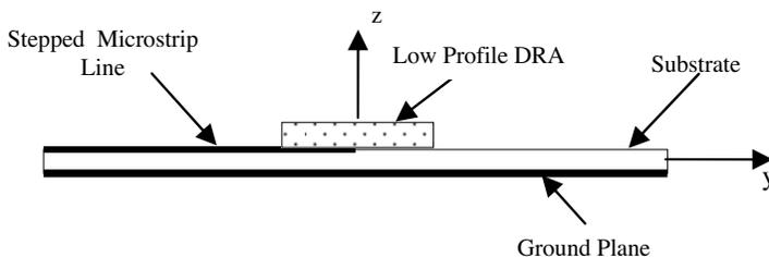
**Figure 1.** Low profile DRA with stepped microstrip feed.
