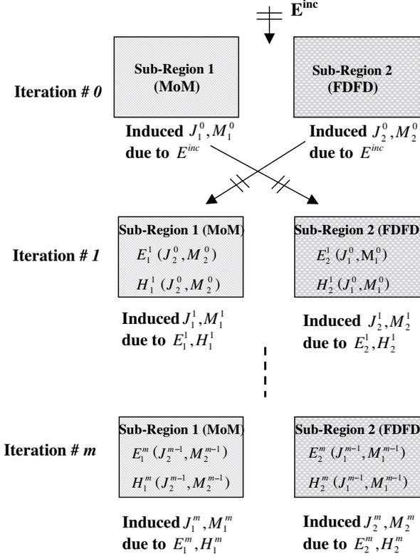
**Figure 2.** Scheme for the iterative procedure applied by converting the electric and magnetic currents to field components generated on the other region.
