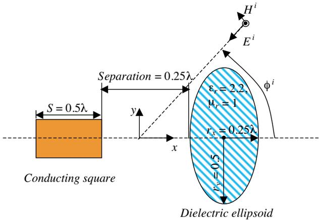
**Figure 5.** Geometry of a conducting square and a dielectric ellipsoid.
