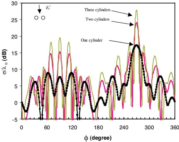
**Figure 10.** Scattering cross section of three different number: one, two, three metamaterial cylinders located on  $x$ -axis with  $3\lambda_0$  center separation and  $a = 1\lambda_0$  radius, metamaterial ( $\epsilon_r = -4$ ,  $\mu_r = -1$ ). The angle of incidence is 90 degrees.
