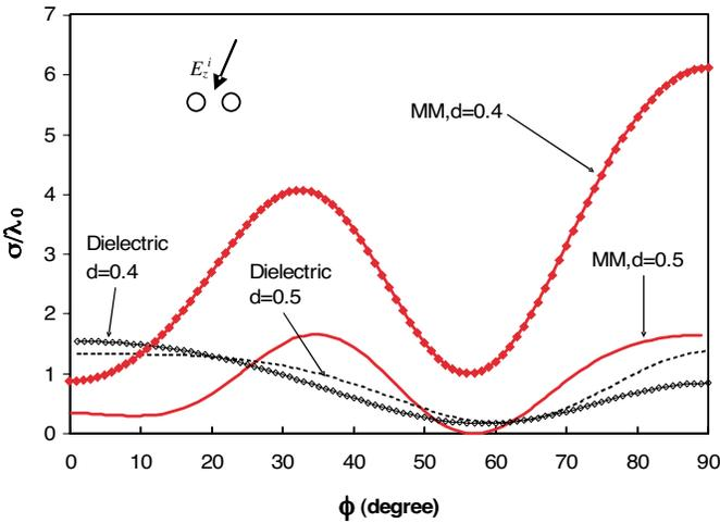
**Figure 5.** Back-scattering cross section versus incidence angle. The configuration includes two cylinders both with  $0.1 \lambda_0$  radius, located on the  $x$ -axis with two different center separation  $0.4 \lambda_0$  and  $0.5 \lambda_0$  and for two cases metamaterial with  $\epsilon_r = -4$ ,  $\mu_r = -1$  and conventional dielectric with  $\epsilon_r = 4$  and  $\mu_r = 1$ .
