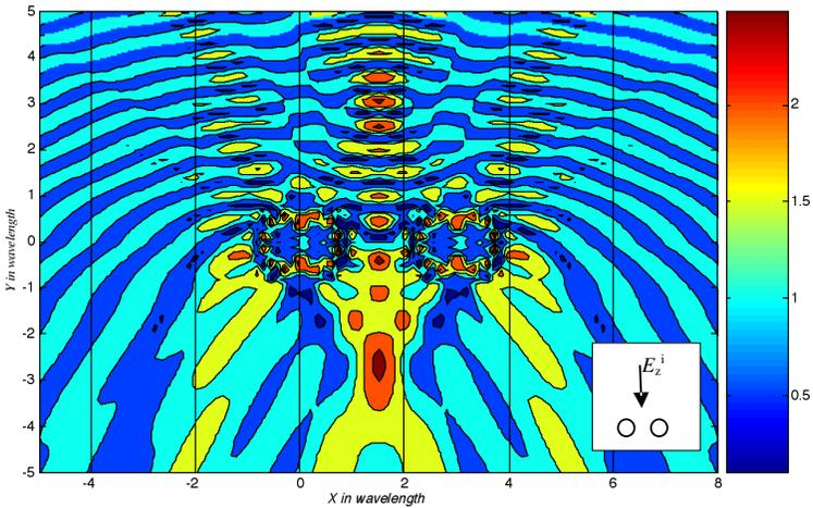
**Figure 9.** Total electric field of two dielectric cylinders located on  $x$ -axis  $x = 0, 3 \lambda_0$  and  $a = 1 \lambda_0$  radius, metamaterial ( $\epsilon_r = -4$ ,  $\mu_r = -1$ ). The angle of incidence is 90 degrees as the small figure in right hand shows.
