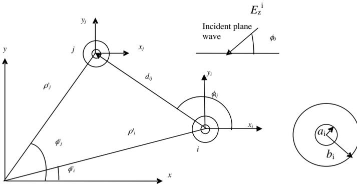
**Figure 1.** Geometry of  $M$  coated cylinders and their local coordinates. Each cylinder defined by radius of conducting cylinder  $a_i$ , radius of coated dielectric or meta-material  $b_i$  and its permeability and permittivity  $(\mu_i, \epsilon_i)$ . Angle Incident plane wave is  $\phi_0$ .
