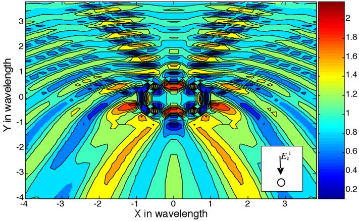
**Figure 8.** Total electric field of one metamaterial cylinder located on  $x$ -axis  $x=0$  with radius  $a = 1 \lambda_0$ , metamaterial ( $\epsilon_r = -4$ ,  $\mu_r = -1$ ). The angle of incidence is 90 degrees as the small figure in right hand shows.
