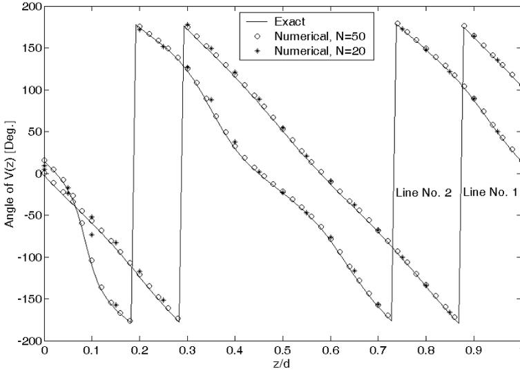
**Figure 5.** The angle of the voltage of uniform coupled transmission lines at frequency of  $f = 1.0$  GHz, obtained from exact formulas and from the proposed method with  $N = 20$  and  $N = 50$  sections.
