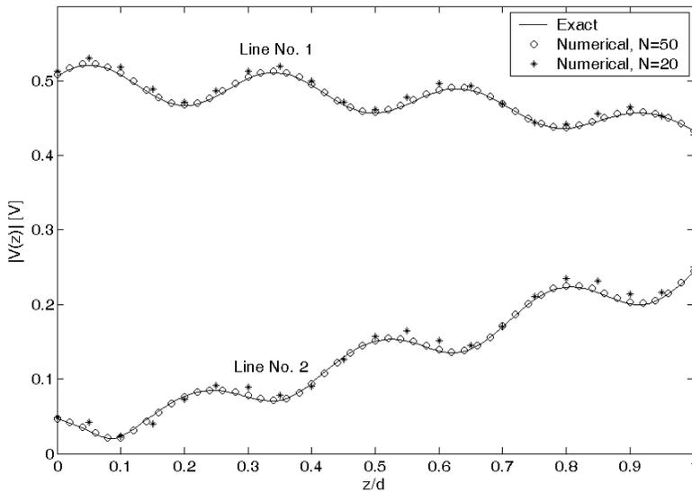
**Figure 4.** The amplitude of the voltage of uniform coupled transmission lines at frequency of  $f = 1.0 \text{ GHz}$ , obtained from exact formulas and from the proposed method with  $N = 20$  and  $N = 50$  sections.
