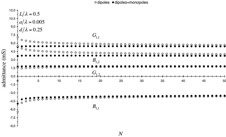
**Figure 2.** Computed self- and mutual admittance of two identical non-staggered dipoles versus  $N$  ( $L/\lambda = 0.5$ ,  $a/\lambda = 0.005$ ,  $d/\lambda = 0.025$ ).
