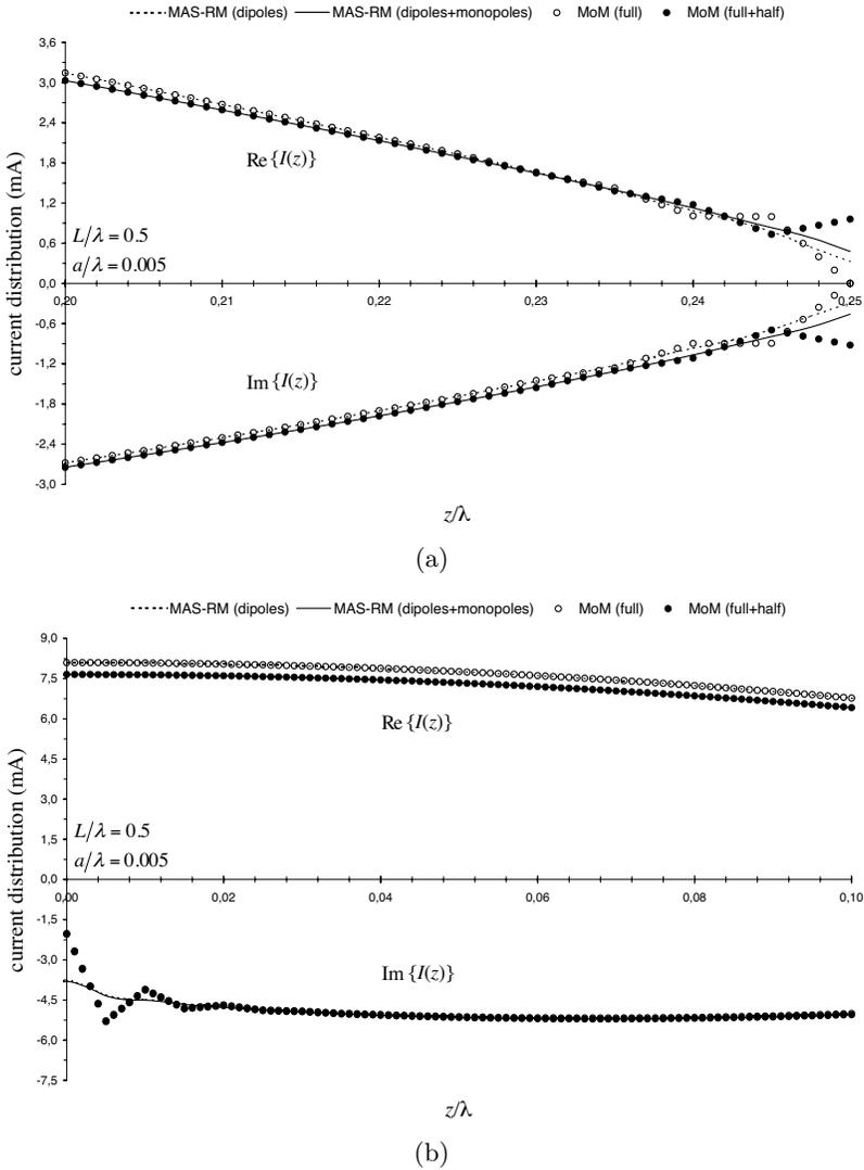
**Figure 3.** Computed current distribution on a symmetrically driven isolated dipole ( $L/\lambda = 0.5$ ,  $a/\lambda = 0.005$ ,  $N + 1 = 50$ ). (a). Current distribution near the ends. (b). Current distribution near the driving point.
