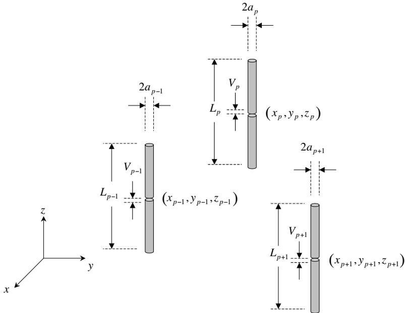
**Figure 1.** General arrangement of arbitrarily located parallel dipoles.
