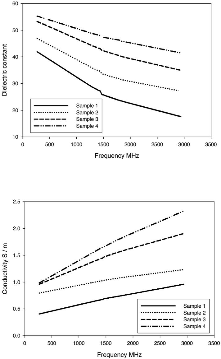
**Figure 2.** Variation of dielectric parameters with frequency for corn syrup samples in the frequency range of 250 MHz–3000 MHz.
