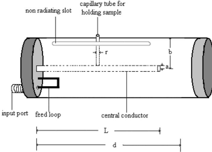
**Figure 1.** Schematic diagram of the coaxial cavity resonator.
