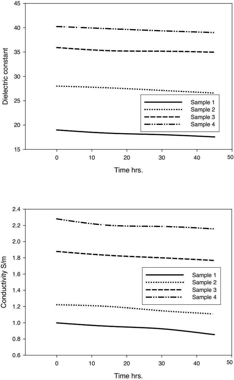
**Figure 3.** Variation of dielectric parameters with time for various corn syrup samples measured at 3000 MHz.
