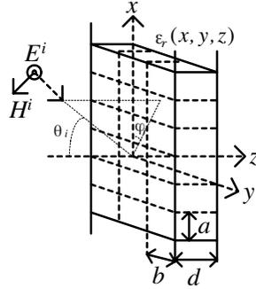
**Figure 1.** A typical grating illuminated by a plane wave.
