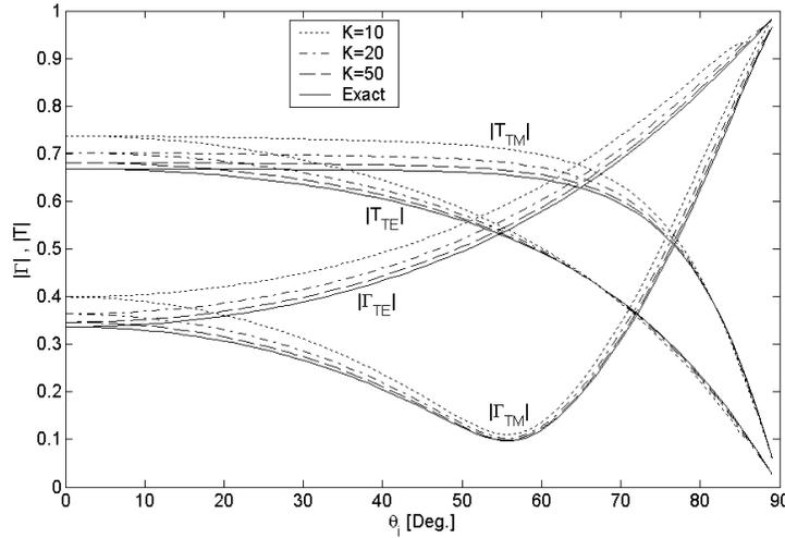
**Figure 2.** The amplitude of the reflection and transmission coefficients of open-end homogeneous planar layer versus  $\theta_i$ .
