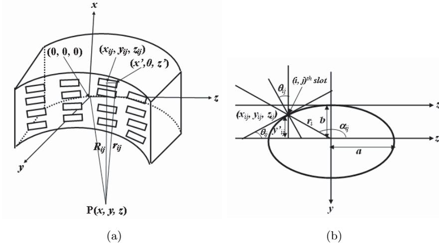
**Figure 1.** (a) Elliptically bent conformal array of longitudinal slots in narrow wall of water-loaded rectangular waveguide (b) angular position and angular orientation of  $(i, j)$ th slot of the conformal array.
