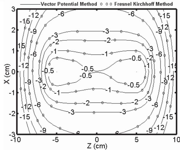
**Figure 2.** Relative SAR contour (in dB) in  $x$ - $z$  plane at  $y = 3.5$  cm for elliptically bent conformal coherent array.
