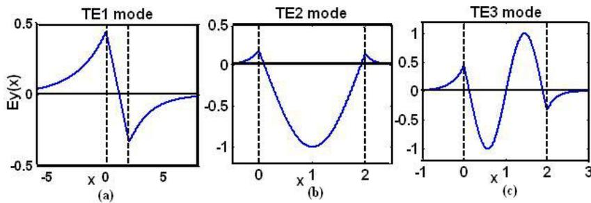
**Figure 3.** Distribution of amplitudes of electric field components of guided modes, where (a)  $V = 1.1363$  (b)  $V = 10$  (c)  $V = 10$ .  $m$  represents the number of intersections between the fields and the  $x$ -axis in region 2.
