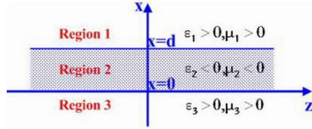
**Figure 1.** Geometry for an asymmetric LHM slab waveguide. Region 2 is LHM, regions 1 and 3 are normal dielectrics.
