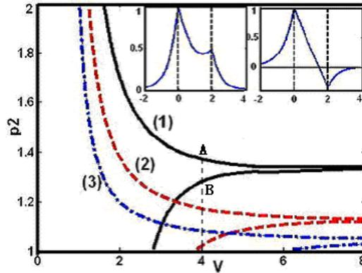
**Figure 5.** Normalized dispersion curves of the surface wave modes with  $n_1 = 1$ ,  $n_2 = -2$ ,  $n_3 = \sqrt{2}$  where (1)  $-\mu_2/\mu_3 = 0.5$  (2)  $-\mu_2/\mu_3 = 1/3$  (3)  $-\mu_2/\mu_3 = 0.2$ . The subgraph represents the distribution of amplitudes of electric field.
