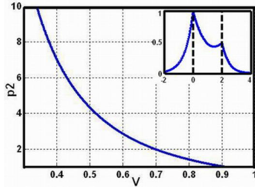
**Figure 4.** Normalized dispersion curve of the surface wave modes with  $\epsilon_1 = 1$ ,  $\mu_1 = 1$ ,  $\epsilon_2 = -2$ ,  $\mu_2 = -2$ ,  $\epsilon_3 = 2$ ,  $\mu_3 = 1$ ,  $d = 2$  cm. The subgraph represents the distribution of amplitudes of electric field.
