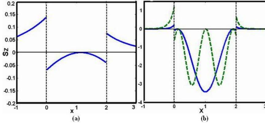
**Figure 7.** Distribution of energy flux along the transverse profile of waveguide for a given waveguide parameters, where (a)  $TE_1$ :  $V = 1.1363$  (b) the dashed line is  $TE_2$ , the real line is  $TE_3$ :  $V = 10$ .
