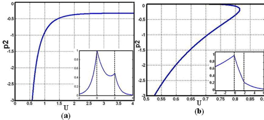
**Figure 6.** Normalized dispersion relationship of the surface wave modes with  $n_1 = 1$ ,  $n_2 = -\sqrt{2}$ ,  $n_3 = 2$ , (a)  $-\mu_2/\mu_3 = 2$  (b)  $-\mu_2/\mu_3 = 0.5$ . The subgraph represents the distribution of amplitudes of electric field.
