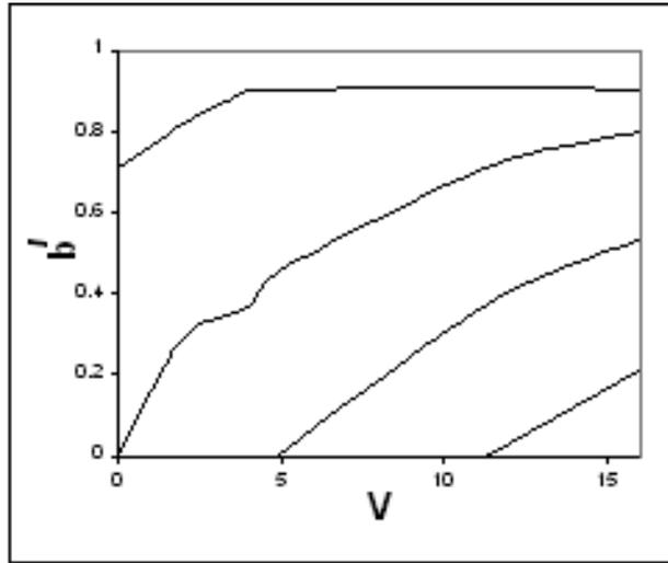
**Figure 9.** Dispersion curves of normalized frequency  $V$  versus normalized propagation constant  $b'$  for the four layered cladding regions with its thickness  $b = 1.0\mu\text{m}$  (hypocycloidal Bragg waveguide).
