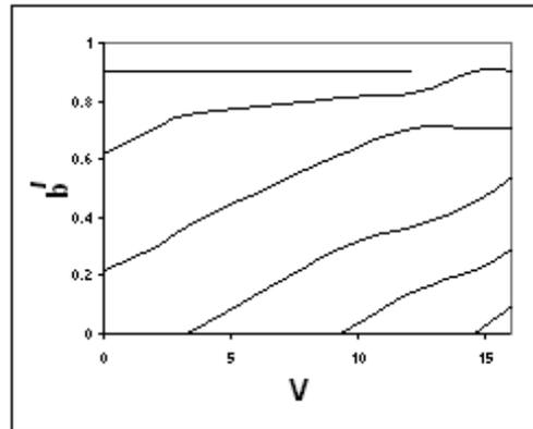
**Figure 8.** Dispersion curves of normalized frequency  $V$  versus normalized propagation constant  $b'$  for the six layered cladding regions with its thickness  $b = 1.0\mu\text{m}$  (hypocycloidal Bragg waveguide).
