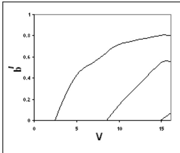
**Figure 6.** Dispersion curves of normalized frequency  $V$  versus normalized propagation constant  $b'$  for the four layered cladding regions with its thickness  $b = 0.10\mu\text{m}$  (hypocycloidal Bragg waveguide).
