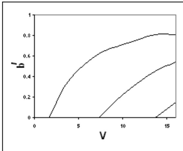
**Figure 10.** Dispersion curves of normalized frequency  $V$  versus normalized propagation constant  $b'$  for the two layered cladding regions with its thickness  $b = 1.0\mu\text{m}$  (hypocycloidal Bragg waveguide).
