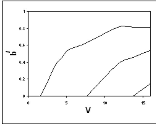
**Figure 5.** Dispersion curves of normalized frequency  $V$  versus normalized propagation constant  $b'$  for the six layered cladding regions with its thickness  $b = 0.10\mu\text{m}$  (hypocycloidal Bragg waveguide).
