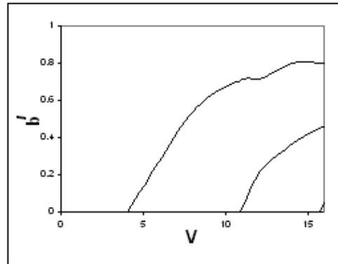
**Figure 3.** Dispersion curves of normalized frequency  $V$  versus normalized propagation constant  $b'$  for the four layered cladding regions with its thickness  $b = 0.01\mu\text{m}$  (hypocycloidal Bragg waveguide).
