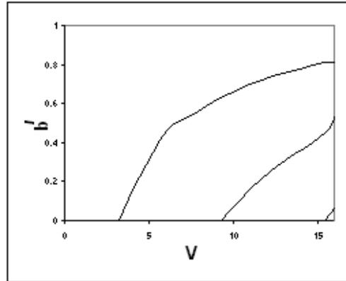
**Figure 7.** Dispersion curves of normalized frequency  $V$  versus normalized propagation constant  $b'$  for the two layered cladding regions with its thickness  $b = 0.10\mu\text{m}$  (hypocycloidal Bragg waveguide).
