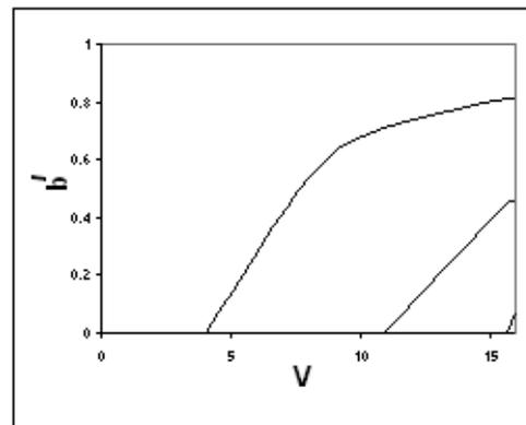
**Figure 4.** Dispersion curves of normalized frequency  $V$  versus normalized propagation constant  $b'$  for the two layered cladding regions with its thickness  $b = 0.01\mu\text{m}$  (hypocycloidal Bragg waveguide).
