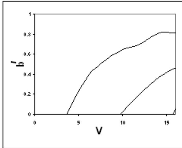
**Figure 2.** Dispersion curves of normalized frequency  $V$  versus normalized propagation constant  $b'$  for the six layered cladding regions with its thickness  $b = 0.01\mu\text{m}$  (hypocycloidal Bragg waveguide).
