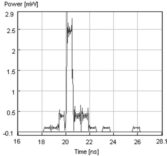
**Figure 6.** Correlator output with fiber included.
