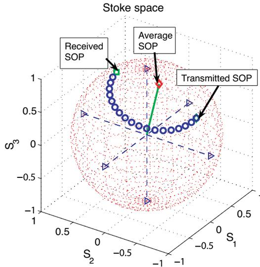
**Figure 3.** Rotation of arbitrarily received SOP to the reference SOP around the average SOP.
