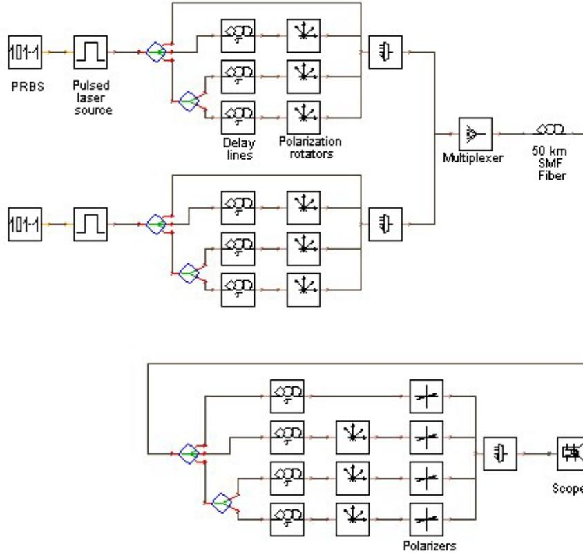
**Figure 4.** VPI simulation setup for two-user Polarized-OOC.
