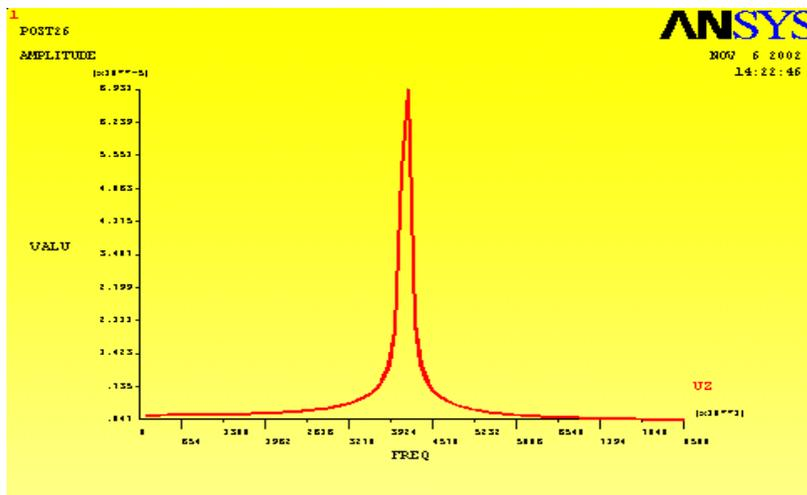
Figure 4. The resonant frequency of the membrane [ $f_{res} = 42.5$  KHz].
