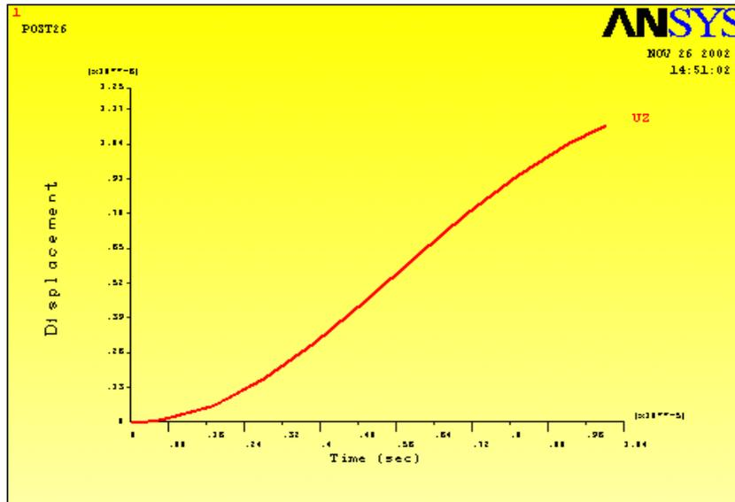
**Figure 5.** Device switching time diagram. The required time for a membrane to displace half the initial separation between the membranes ( $0.75 \mu\text{m}$ ) is  $6.5 \mu\text{sec}$ .
