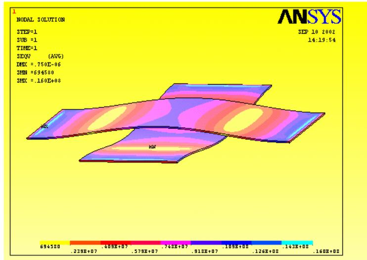
Figure 3. Stress distribution on the double membranes structure.
