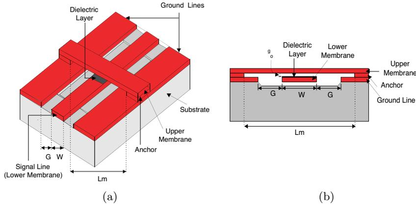
**Figure 1.** Schematic diagram of our Proposed Switch: (a) a 3D isometric view of the switch; (b) the cross-sectional view of the switch  $Lm = 280 \mu\text{m}$ .
