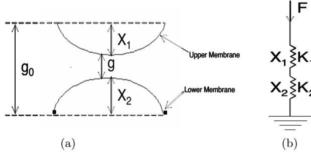
**Figure 2.** The displacement of the membranes.
