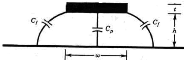
**Figure 2.** Capacitance model for stripline transmission line [10].
