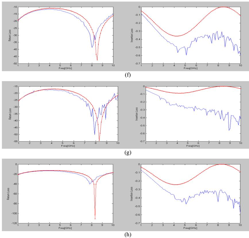
**Figure 4.** The comparison of scattering matrix of the model, regardless of the radiation resistance, with HFSS simulation.  $w/h =$  (a) 0.813 (b) 0.976 (c) 1.301 (d) 2.276 (e) 2.602 (f) 3.252 (g) 3.577 (h) 4.065.
