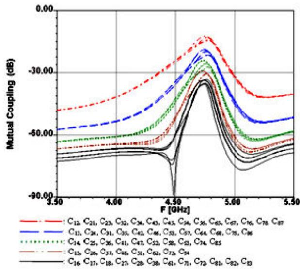
Figure 11. Mutual Coupling of proposed fractal patch array.
