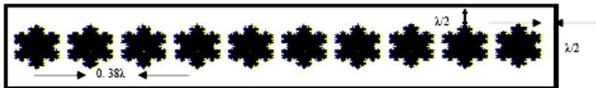
**Figure 3.** The structure of proposed fractal patch array.
