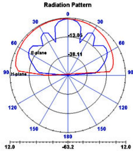
Figure 10. Radiation pattern of proposed fractal patch array in *E* and *H* planes.
