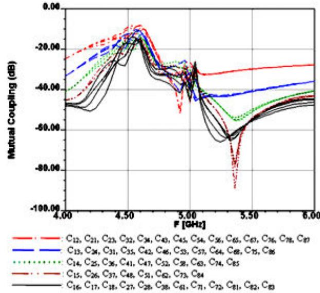
Figure 12. Mutual Coupling of conventional rectangular patch array.
