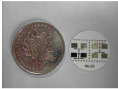
Figure 10. Photograph of the improved MADA.
