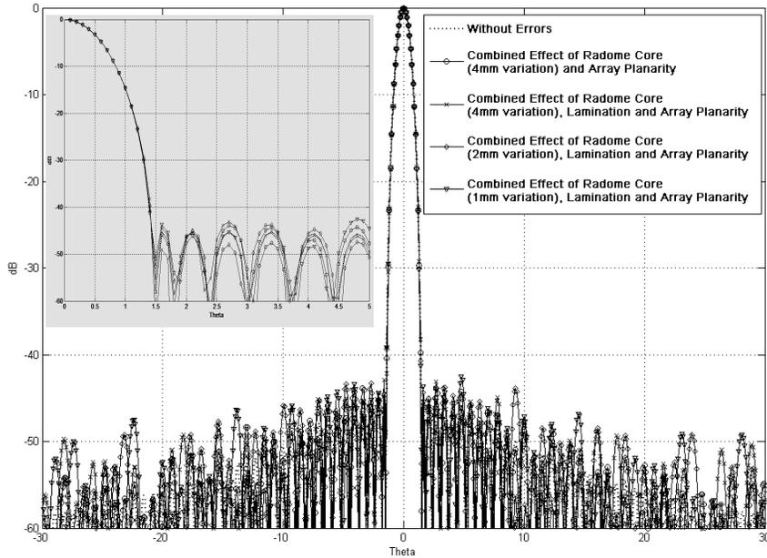
**Figure 12.** Combined effect of variations in characteristics of multilayer flat sandwich radome (with different core thickness), 6 bit amplitude/phase quantisation error and array planarity error on active phased array antenna radiation pattern (exploded view of one half of the pattern is shown as an inset).
