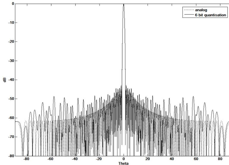
**Figure 2.** Effect of 6 bit amplitude quantisation on far-field radiation pattern of  $(160 \times 10)$  elements active phased array antenna.
