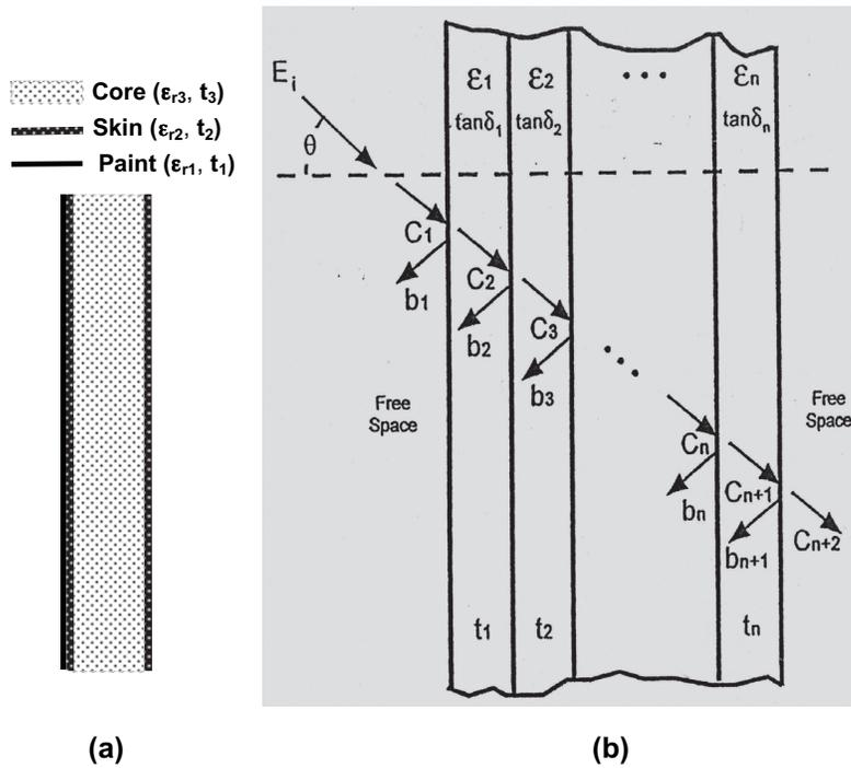
**Figure 5.** Multilayer flat sandwich radome (a). Structural view [ $\epsilon_{r3} = 1.16$ ;  $t_3 = 1000$  mils (25 mm) typically;  $\epsilon_{r2} = 4.25$ ;  $t_2 = 33$  mils (0.84 mm) typically;  $\epsilon_{r1} = 3.65$ ;  $t_1 =$  mils (5 mm) typically] (b). Boundary-value solution of the  $N$ -layer dielectric wall radome.
