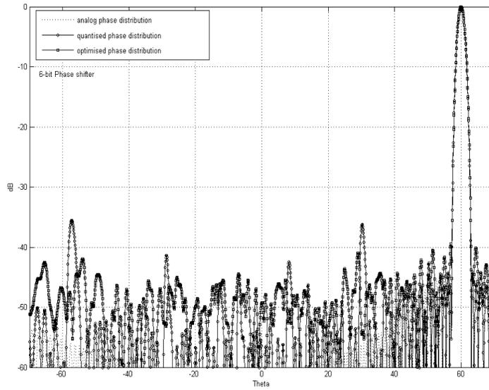
**Figure 3.** Effect of 6 bit phase quantisation with and without optimisation on far-field radiation pattern of  $(160 \times 10)$  elements active phased array antenna.
