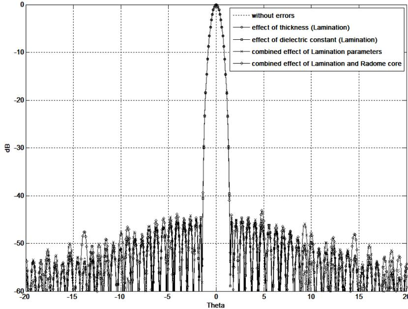
**Figure 11.** Effect of variations in characteristics of lamination layer and core of multilayer flat sandwich radome individually and in combined manner on active phased array antenna radiation pattern.
