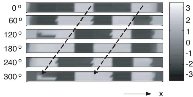
**Figure 5.** Electrical field distribution inside the slab of metamaterial when it reaches steady state. The continuous plane wave at 5 GHz is incident from left. There are six unit cells along the  $\hat{x}$  direction. The arrows with dashed line indicate the phase front propagates along the  $-\hat{x}$  direction.
