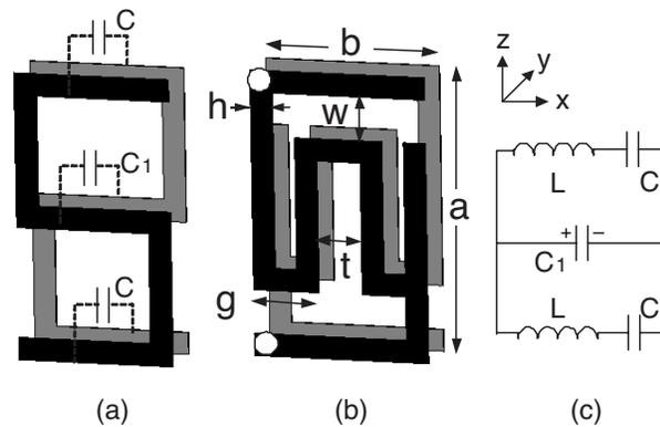
**Figure 1.** (a) S-ring resonator. (b) The cranked S-ring resonator. The effective capacitance  $C_1$  is enlarged by cranking the central metallic strips. The white circles in the top and bottom horizontal strips indicate the positions of the vias. (c) The equivalent circuit for the two rings.
