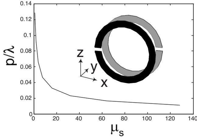
**Figure 7.** Simulated result on the structure size of the broad-side coupled SRR as a function of the permeability of the substrate. The inner radius of the SRR is  $r = 1.6$  mm, the width of the metal strip is  $d = 0.4$  mm, and the thickness of the substrate is  $g = 0.4$  mm. the period of the structure is 6 mm, 1.2 mm and 6 mm in the  $\hat{x}$ ,  $\hat{y}$ , and  $\hat{z}$  directions, respectively.
