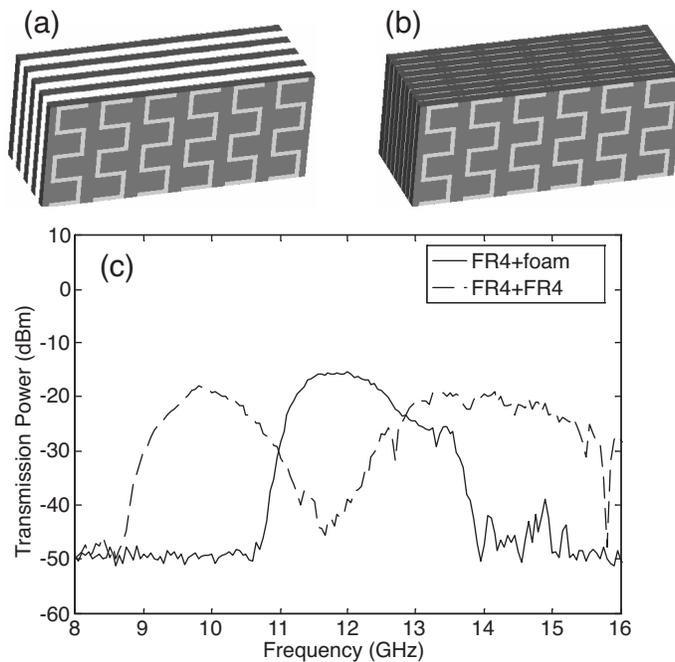
**Figure 6.** (a) SR with FR4+foam structure: layered of the FR4 substrate (dark color) printed with S-shaped resonator are aligned with layered of foam slice (white color). (b) SR with FR4+FR4 structure: layered of the FR4 substrate printed with SR are aligned with layered of empty FR4 substrate. (c) Transmission results for the two metamaterials.
