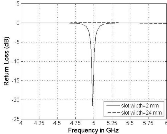
**Figure 2.** Return loss for the CPW-fed narrow and wide slots.
