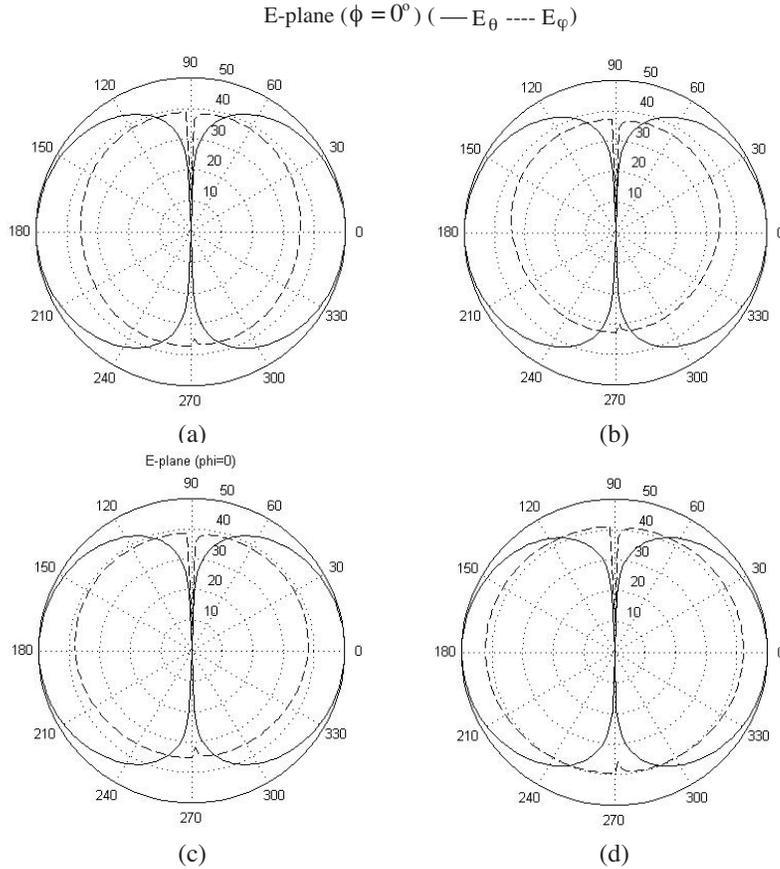
**Figure 9.**  $E$ -plane ( $\phi = 0^\circ$ ) radiation patterns for wide slot with inverted F-shaped stub, (a) Frequency=1.2 GHz, (b) Frequency=1.5 GHz, (c) Frequency=1.35 GHz, (d) Frequency=1.65 GHz.
