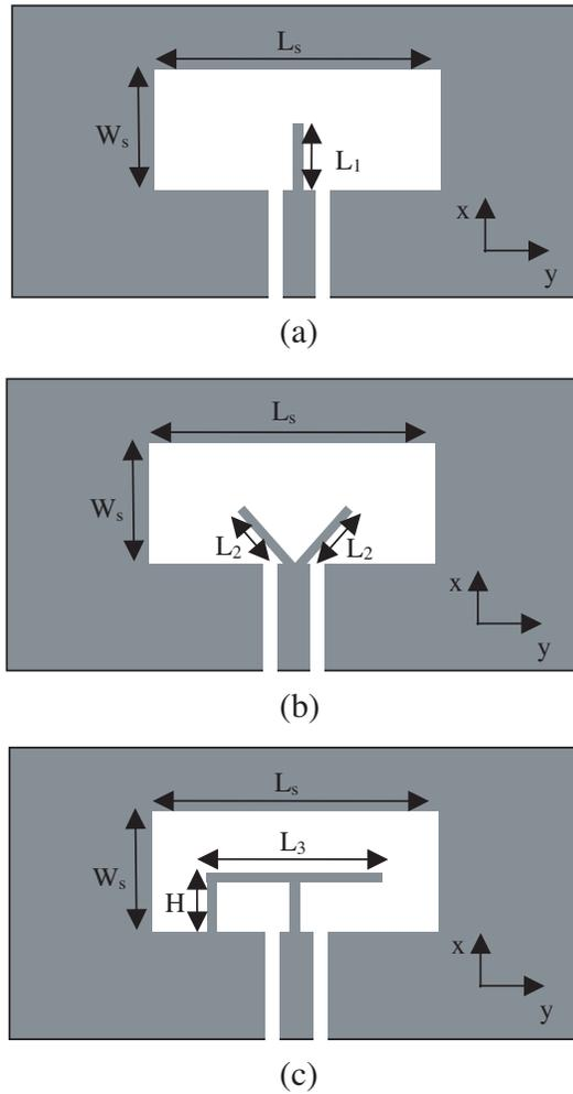
**Figure 3.** CPW-fed wide slot with various tuning stubs (slot dimensions:  $L_s = 48$  mm,  $W_s = 24$  mm), (a) single straight stub in a wide slot, (b) V-shaped stub in a wide slot, (c) inverted F-shaped stub in a wide slot.
