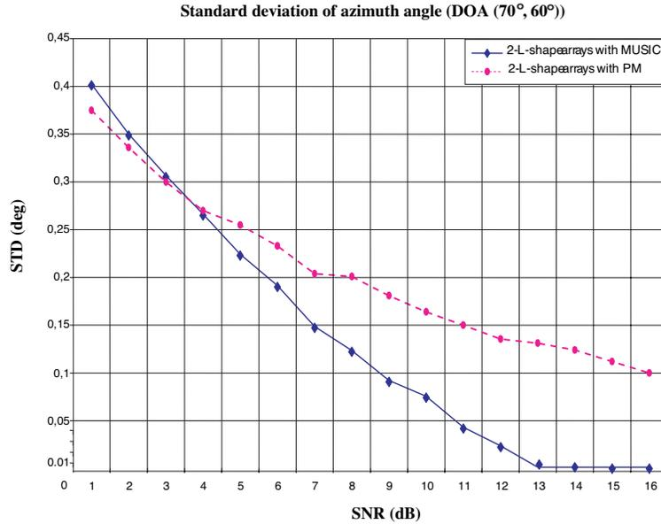
**Figure 6.** Standard deviation of the azimuth angle estimation versus SNR for a single source at  $(70^\circ, 60^\circ)$  using both the PM method in [8] and the proposed MUSIC of the 2-L-shape arrays.
