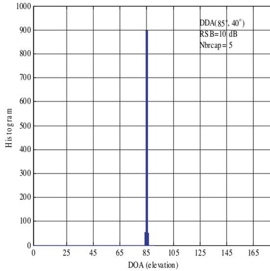
**Figure 4.** Histogram of elevation DOA estimations for a single source of DOA at  $(85^\circ, 40^\circ)$   $SNR = 10$  dB,  $N = 5$  elements by using the proposed MUSIC of the 2-L-shape arrays configuration.
