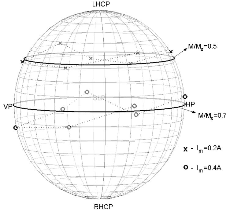
**Figure 5.** Experimental and simulated polarization state parameters of the wave at the output of the ferrite section for LHCP input, evaluated versus  $\theta$  and selected two values of magnetization currents  $I_m$  ( $M/M_s$ ) (ferrite rod parameters, radius  $a = 18.59$  mm, length  $z = 98$  mm,  $M_s = 250$  Gauss,  $\epsilon_r = 13.5$ ).
