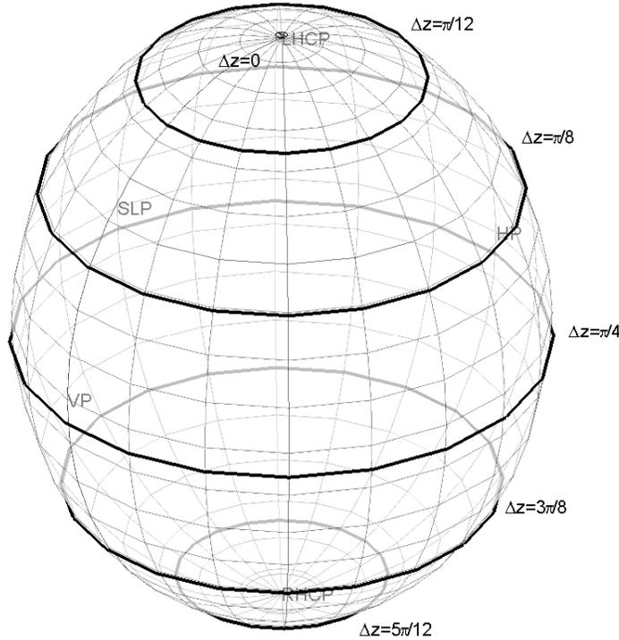
**Figure 4.** Polarization states of the output wave for input LHCP wave defined by points on circles evaluated versus  $\theta$  for selected values  $\Delta \cdot z$  and performed on Poincare sphere.
