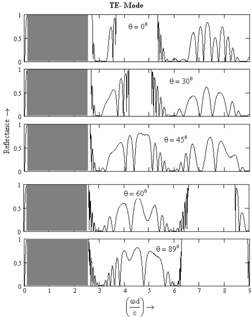
**Figure 5a.** Reflectance curve for PC2 structure having  $n_1 = 1.35$  and  $n_2 = -3.6$  and layer thickness  $d_1 = 0.7d$  and  $d_2 = 0.3d$  respectively for both TE and TM polarizations respectively.
