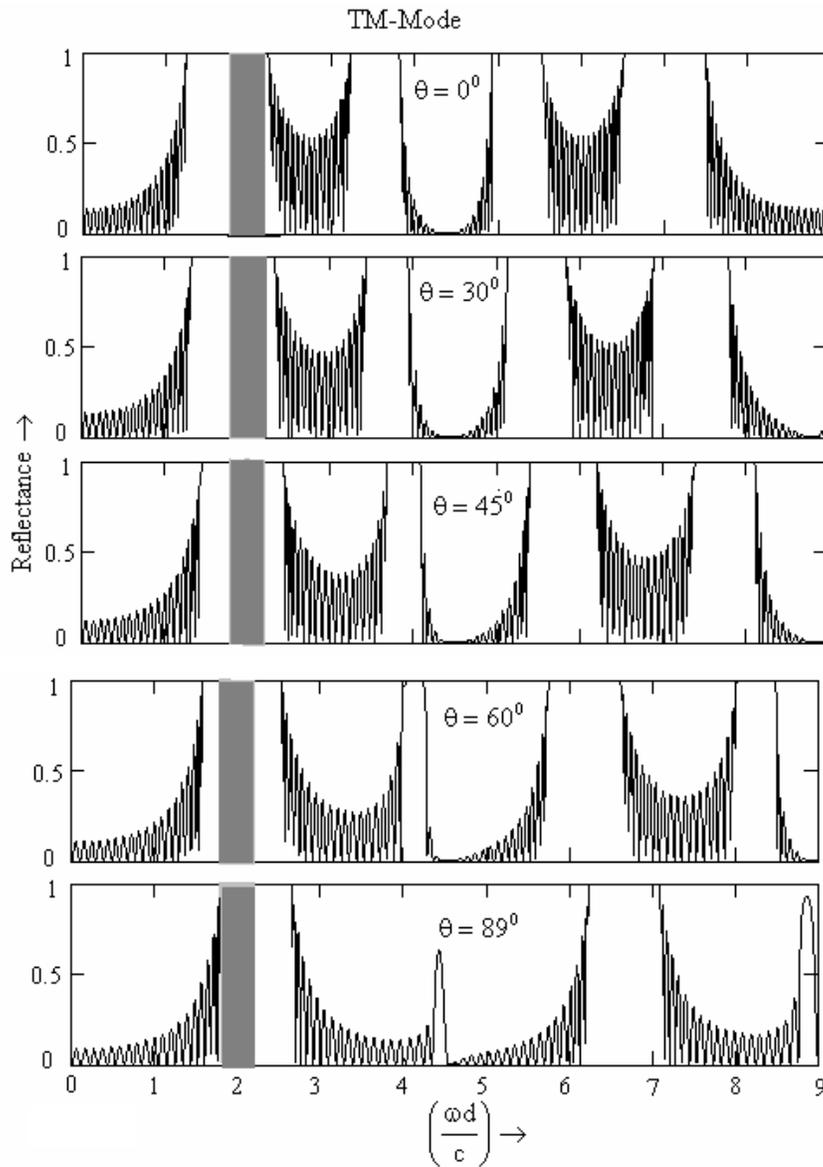
**Figure 4b.** Reflectance curve for PC1 structure having  $n_1 = 1.35$  and  $n_2 = 3.6$  and layer thickness  $d_1 = 0.8d$  and  $d_2 = 0.2d$  respectively for both TE and TM polarizations respectively.
