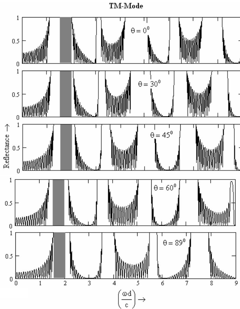
**Figure 6b.** Reflectance curve for PC1 structure having  $n_1 = 1.35$  and  $n_2 = 3.6$  and layer thickness  $d_1 = 0.7d$  and  $d_2 = 0.3d$  respectively for both TE and TM polarizations respectively.
