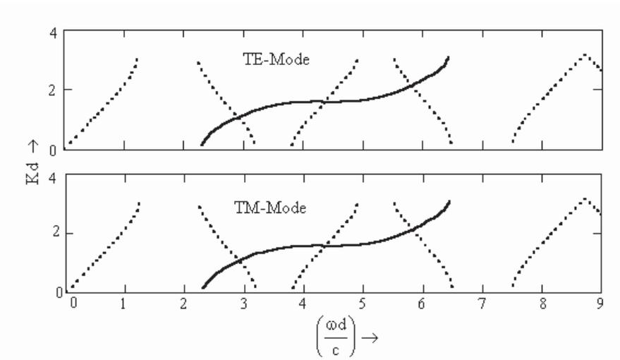
**Figure 2a.** The plot of dispersion relation for PC1 ( $n_1 = 1.35$  and  $n_2 = 3.6$ ) PC2 ( $n_1 = 1.35$  and  $n_2 = -3.6$ ) structure with layer thickness  $d_1 = 0.8d$  and  $d_2 = 0.2d$  respectively for both TE and TM modes. Dotted line is used for PC1 and solid line is used for PC2.
