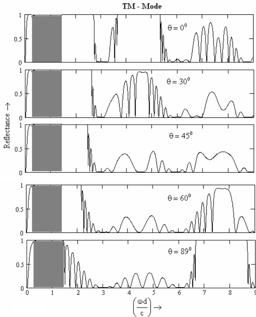
**Figure 5b.** Reflectance curve for PC2 structure having  $n_1 = 1.35$  and  $n_2 = -3.6$  and layer thickness  $d_1 = 0.7d$  and  $d_2 = 0.3d$  respectively for both TE and TM polarizations respectively.
