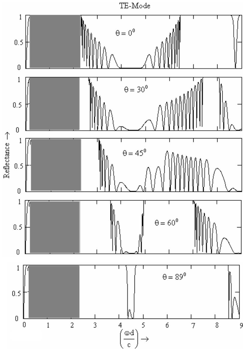
**Figure 3a.** Reflectance curve for PC2 structure having  $n_1 = 1.35$  and  $n_2 = -3.6$  and layer thickness  $d_1 = 0.8d$  and  $d_2 = 0.2d$  respectively for both TE and TM polarizations respectively.
