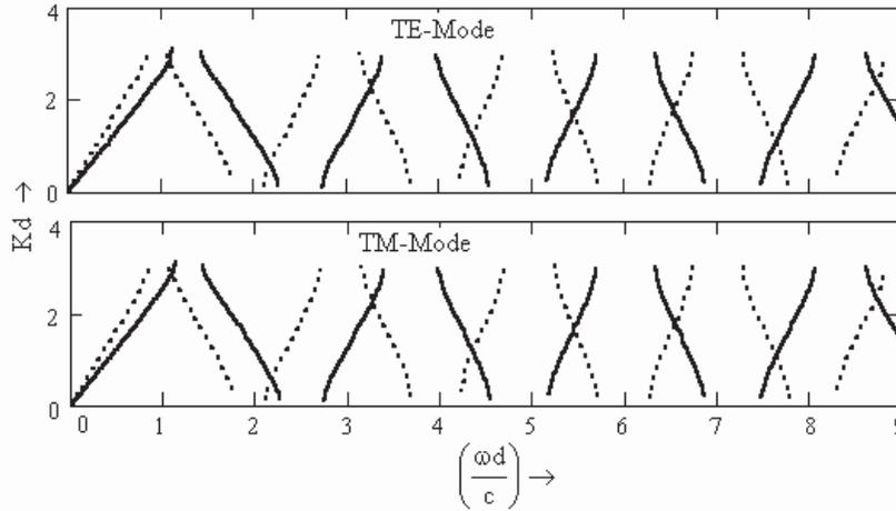
**Figure 2b.** The plot of dispersion relation for PC1 ( $n_1 = 1.35$  and  $n_2 = 3.6$ ) PC2 ( $n_1 = 1.35$  and  $n_2 = -3.6$ ) structure with layer thickness  $d_1 = 0.2d$  and  $d_2 = 0.8d$  respectively for both TE and TM modes. Dotted line is used for PC1 and solid line is used for PC2.
