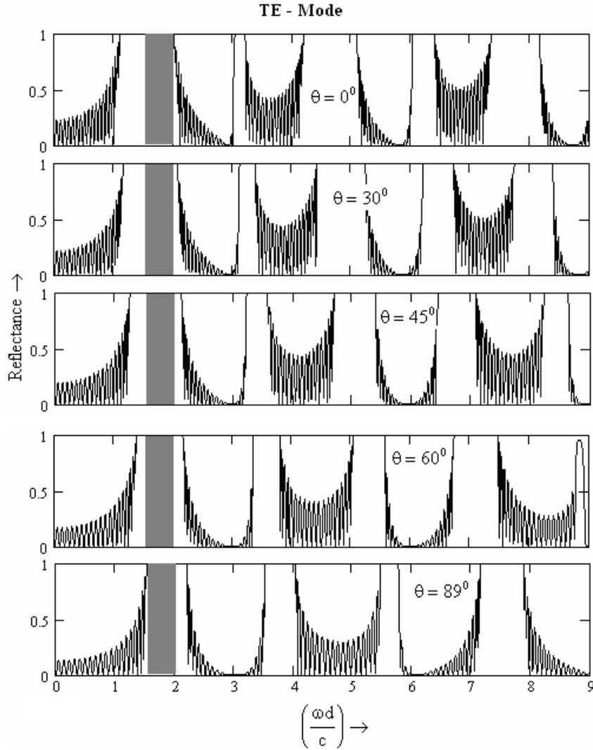
**Figure 4a.** Reflectance curve for PC1 structure having  $n_1 = 1.35$  and  $n_2 = 3.6$  and layer thickness  $d_1 = 0.8d$  and  $d_2 = 0.2d$  respectively for both TE and TM polarizations respectively.
