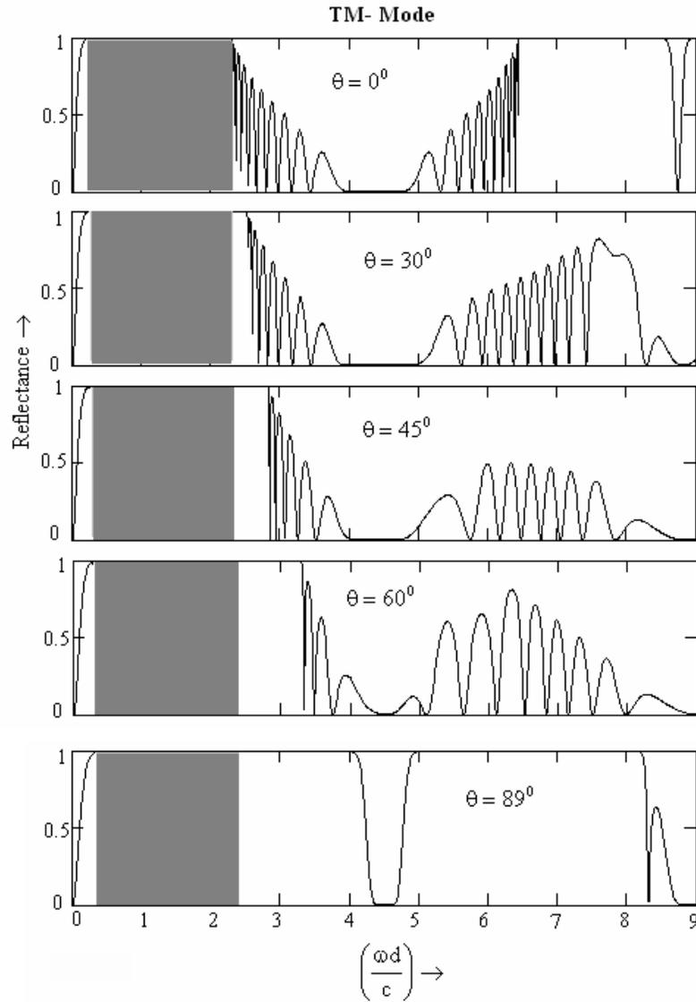
**Figure 3b.** Reflectance curve for PC2 structure having  $n_1 = 1.35$  and  $n_2 = -3.6$  and layer thickness  $d_1 = 0.8d$  and  $d_2 = 0.2d$  respectively for both TE and TM polarizations respectively.
