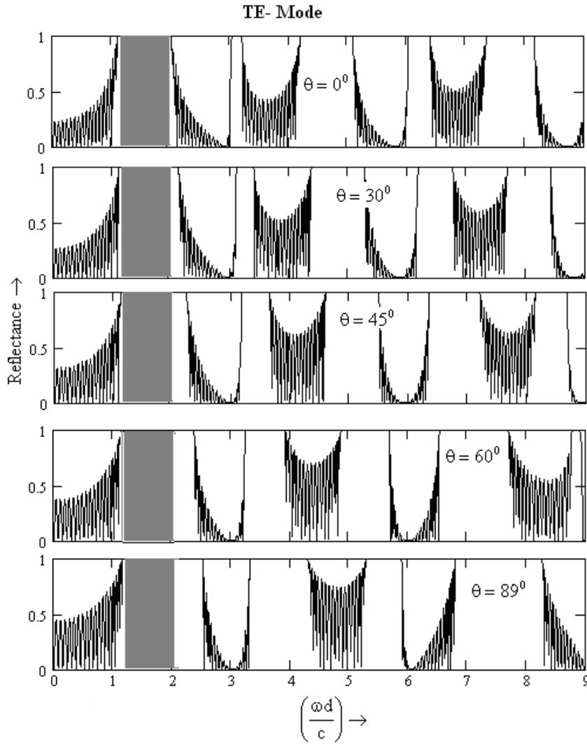
**Figure 6a.** Reflectance curve for PC1 structure having  $n_1 = 1.35$  and  $n_2 = 3.6$  and layer thickness  $d_1 = 0.7d$  and  $d_2 = 0.3d$  respectively for both TE and TM polarizations respectively.
