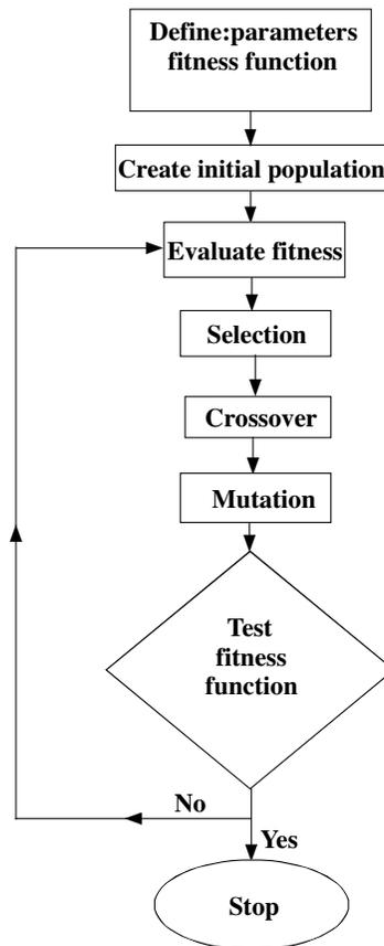
**Figure 2.** Flow chart of floating-point GA.
