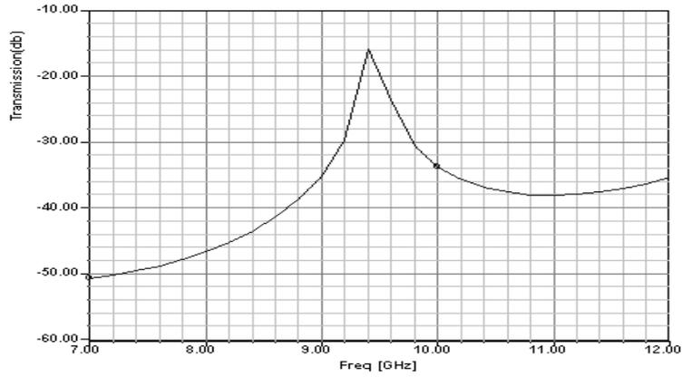
**Figure 3.** Transmission of the lattice of split ring.
