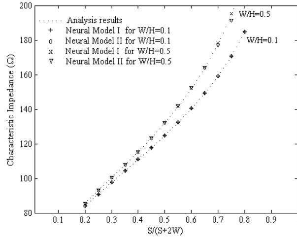
**Figure 5.** Comparisons among the characteristic impedances calculated by using the first synthesis neural model  $Z_0(W, \varepsilon_r, H)$  for a given  $S$ ; the second synthesis neural model  $Z_0(S, \varepsilon_r, H)$  for a given  $W$ ; and the quasi-static analysis [6]  $Z_0(W, S)$ , with  $\varepsilon_r = 10.2$ .
