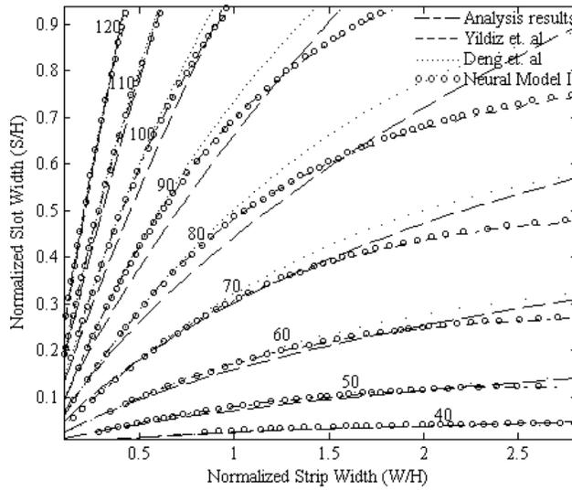
**Figure 3.** Comparisons among the neural synthesis results  $W(Z_0, S)$  using the first neural model, the synthesis results  $W(Z_0, S)$  of Deng et al. [10] and Yildiz et al. [12], and the quasi-static analysis [6] contours of  $Z_0(S, W)$ , with  $\epsilon_r = 12.9$  and  $H = 200 \mu\text{m}$ .
