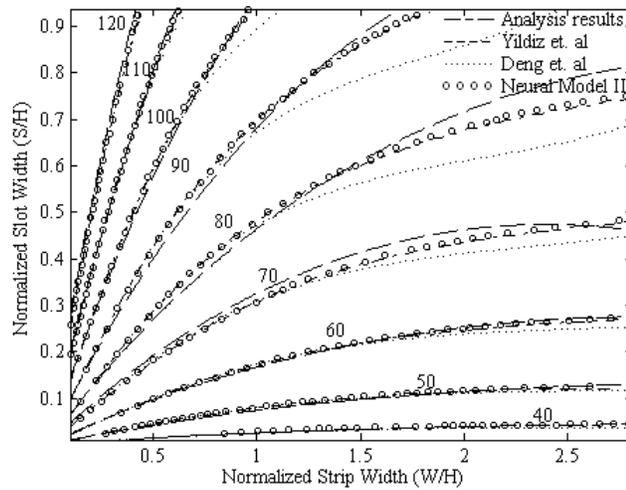
**Figure 4.** Comparisons among the neural synthesis results  $S(Z_0, W)$  using the second neural model, the synthesis results  $S(Z_0, W)$  of Deng et al. [10] and Yildiz et al. [12], and the quasi-static analysis [6] contours of  $Z_0(S, W)$ , with  $\epsilon_r = 12.9$  and  $H = 200 \mu\text{m}$ .
