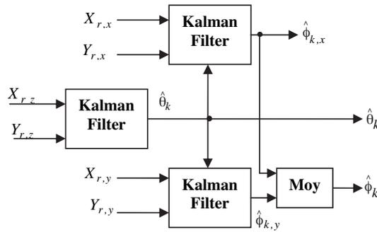
**Figure 2.** Proposed two L-shape array flowchart for the joint elevation and azimuth DOA estimation.
