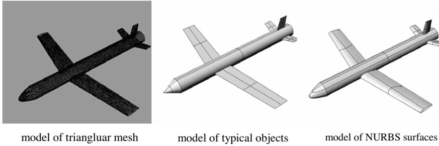
**Figure 1.** A simplified aircraft modeled in different ways.
