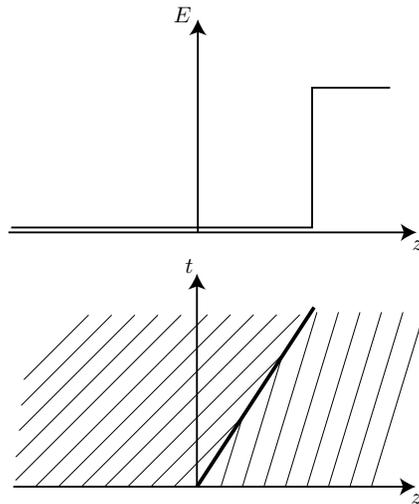
**Figure 2.** Top: the (physical) shock wave (57) for a given time  $t$ . Bottom: the '+'-characteristics corresponding to this solution. Note that the characteristics cross each other on the shock front, indicated by the bold line.
