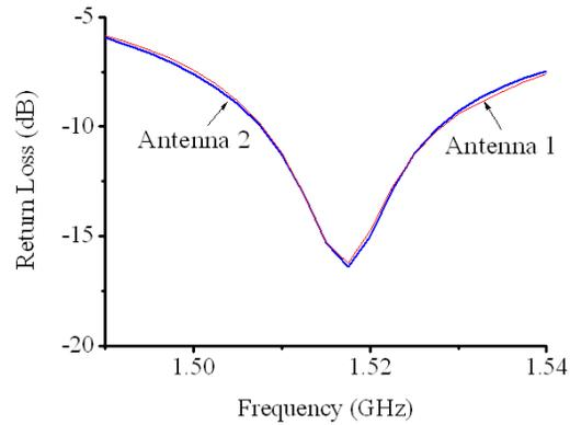
**Figure 3.** Measured return losses of antenna 1 and antenna 2.
