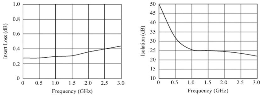
**Figure 2.** Insert loss and isolation of SPDT switch.
