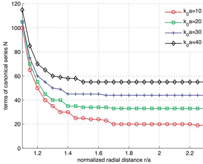
**Figure 2.** The required number of terms  $N$  which are necessary to achieve convergence as function of the normalized radial distance  $r/a$  for various electrical radii of the sphere  $k_0 a$ . The canonical series is the used formula.
