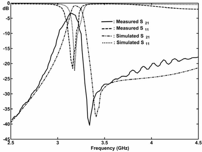
Figure 7. Simulated and measured results of filter 1.
