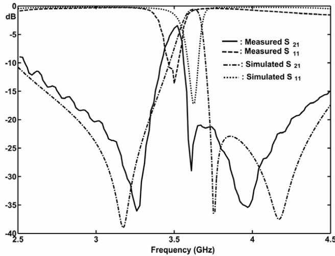
**Figure 9.** Simulated and measured results of filter 2.
