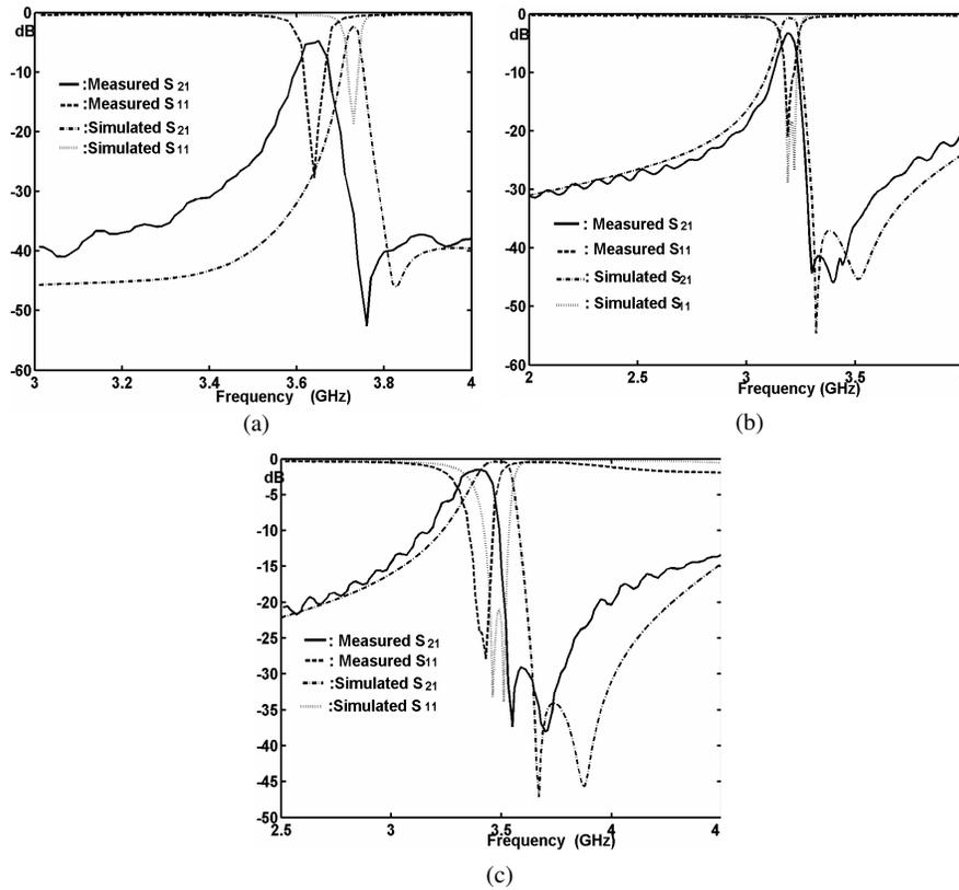
**Figure 3.** Simulated and measured results (a) type 1, (b) type 2, (c) type 3.
