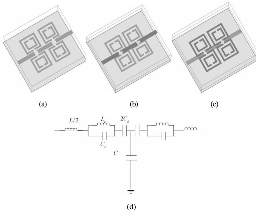
**Figure 2.** Layout of SRRs with coupled line and equivalent circuit model (a) type 1: SRRs coplanar with coupled line, (b) type 2: SRRs below coupled line, (c) type 3: SRRs above coupled line, (d) equivalent circuit model.
