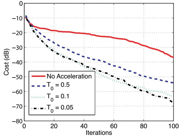
**Figure 6.** Convergence curves for the synthesis of symmetric pattern by using a linear array of 14 elements. The population size is 8 particles. The inertia factor  $w$  is decreased linearly from 0.9 to 0.2.  $c_1 = c_2 = 2.0$ .
