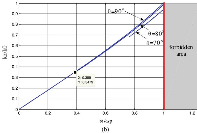
**Figure 3.** Dispersion characteristics for the surface TM modes in case (i): (a) when the direction of the external magnetic field is fixed ( $\theta = 45^\circ$ ); (b) when the parameter ratio is fixed ( $\epsilon_1 \mu_1 / (\epsilon_0 \mu_2) = 0.8$ ). Each case has a cut-off frequency except  $\theta = 90^\circ$ . Shaded area in each figure indicates the frequency domain where the surface waves are forbidden.
