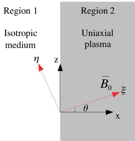
**Figure 1.** Diagram for an interface between a semi-infinite isotropic medium and a uniaxial plasma. The  $\xi$  axis indicates principle axis, also the direction of the external magnetic field which is infinitely strong in the uniaxial plasma.
