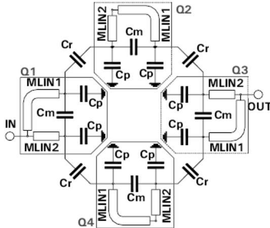
**Figure 2.** Circuit simulator scheme.
