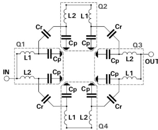
**Figure 1.** Basic electric scheme of proposed filter.
