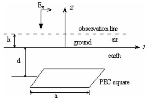
**Figure 3.** PEC square buried under flat plane.
