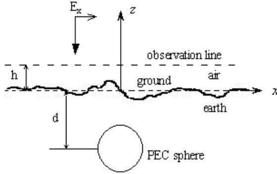
**Figure 7.** PEC sphere buried under random rough surface.
