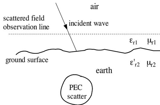
**Figure 1.** PEC object buried under ground surface.
