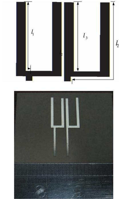
Figure 7. Layout and photograph of two-pole filter.
