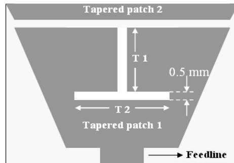
**Figure 9.** Geometry of the tapered patch 1 with a modified T-shaped slot.
