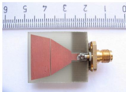
**Figure 5.** Photograph of the realized printed PTMA.
