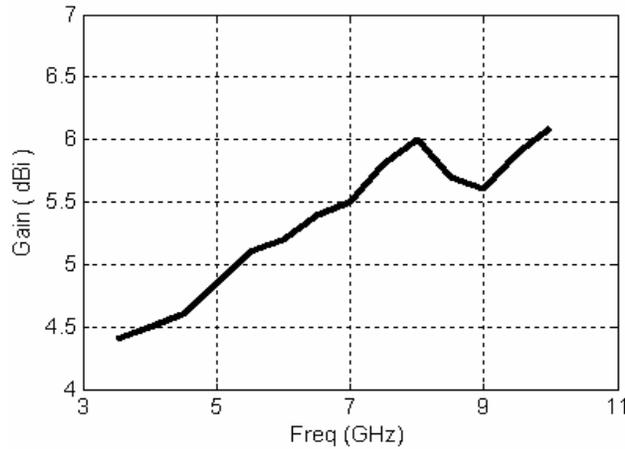
**Figure 7.** Simulated antenna gain of the proposed antenna.
